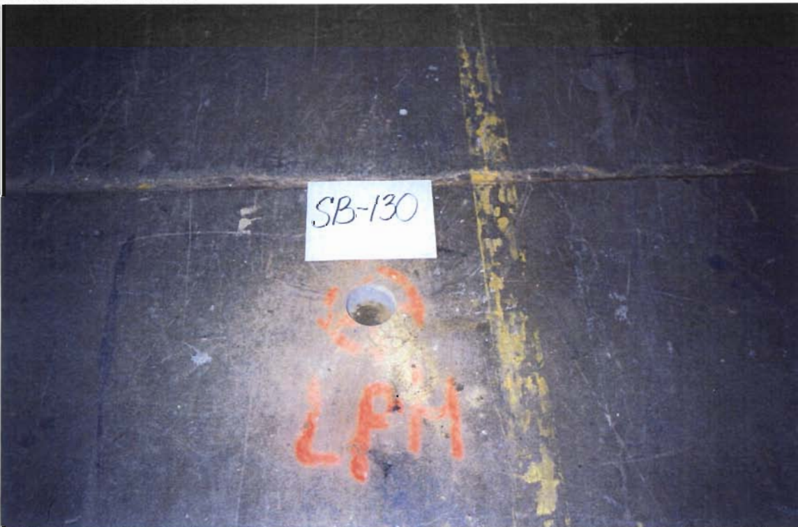
Soil boring SB-130 was placed in the center of the former Gilbert Displays Building, at the location of a former historic leaching pool.
