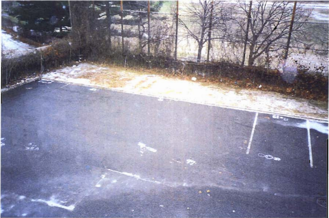
Rear of former Gilbert Displays Building (view from roof). Numbers marked on pavement denote boring locations.
