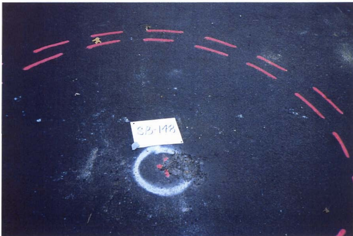
Soil boring SB-148 was advanced to investigate an anomalous area on Air Techniques.
