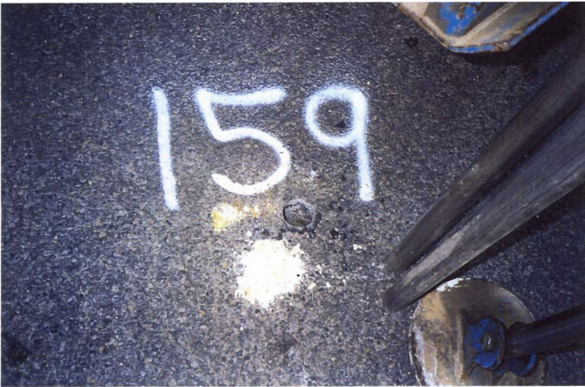
Soil boring SB-159 was advanced to further define the concentrations of contaminants east of and between SB-077 and SB-082.
