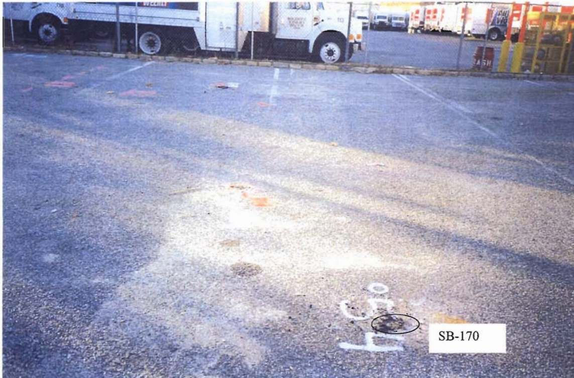
Soil boring SB-170 was advanced at the request of NYSDEC to delineate the building rubble identified in SB-054. There was no rubble identified in SB-170.
