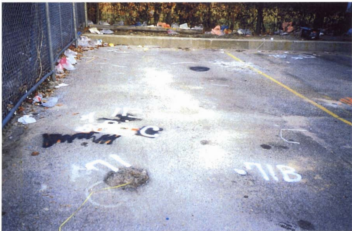
SB-113 A, B, and C. Borings 113B and C were discrete sampling locations. These borings were installed to delineate Nickel in the subsurface at this location.
