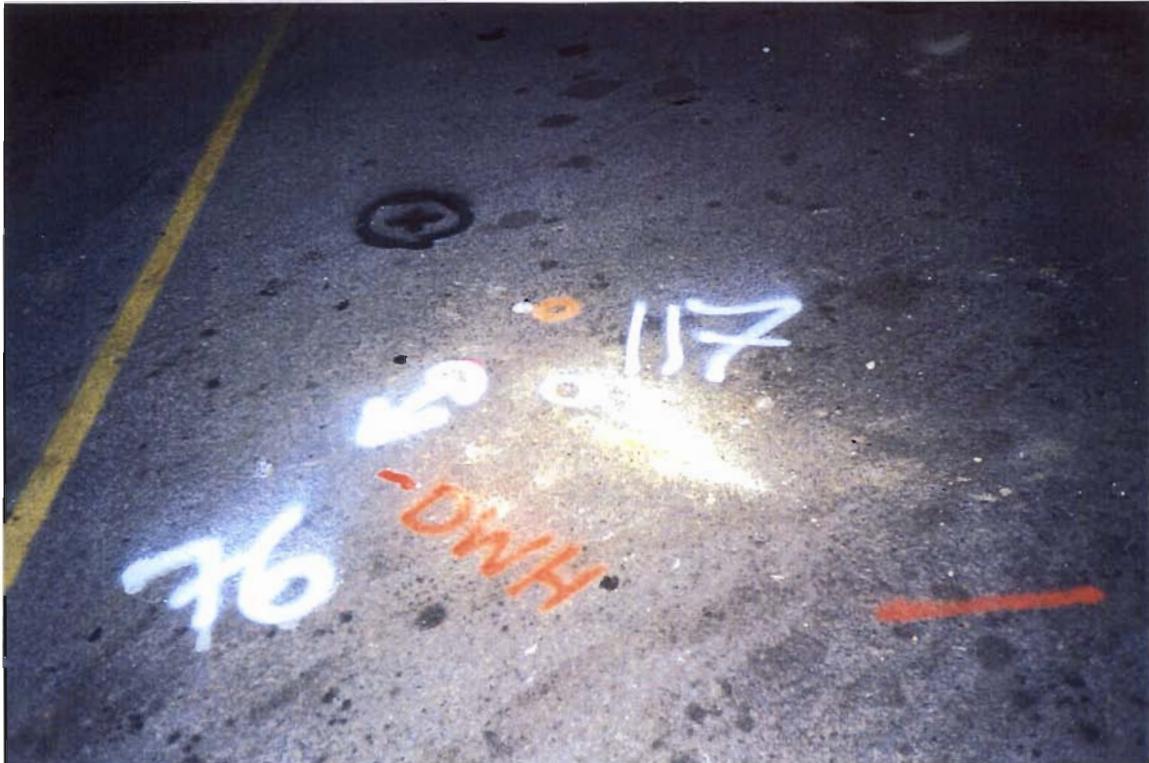
Soil boring SB-117 at the corner of the Magazine Distributors Building at a historic drywell location.
