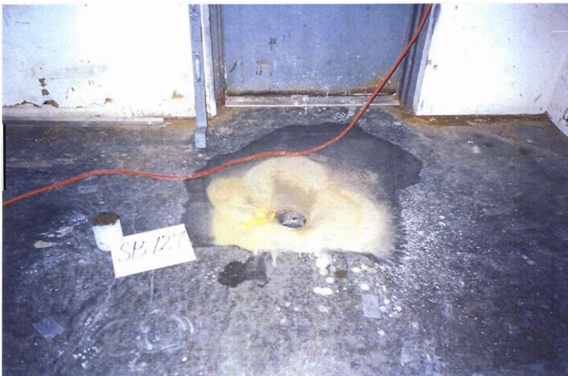
Soil boring SB-127 inside the former Gilbert Displays Building. This location was a supplemental location chosen by Jack Kadelecek, NYSDEC.
