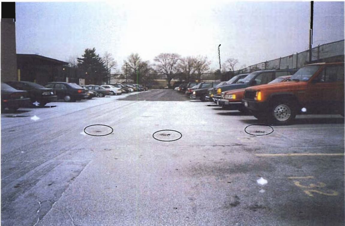
Soil borings SB-163, SB-164, and SB-165 were used to delineate radionuclides in surface materials at Air Techniques.
