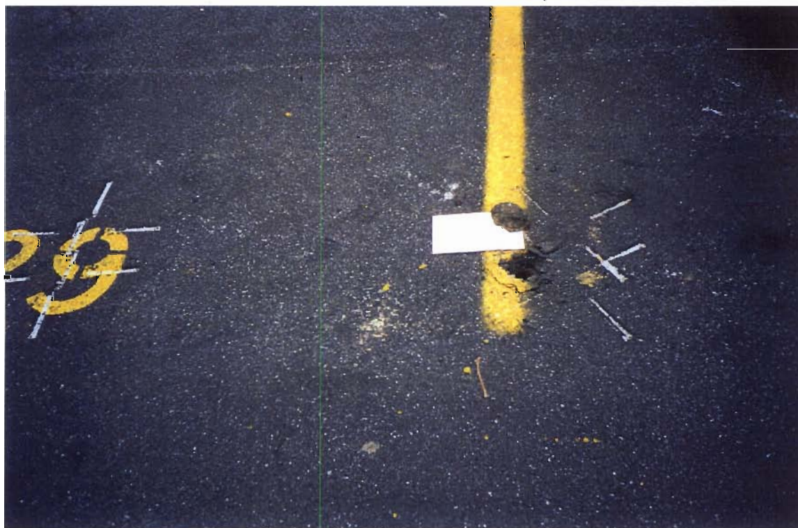
Soil boring SB-162 was used to delineate radionuclides in surface materials at Air Techniques.
