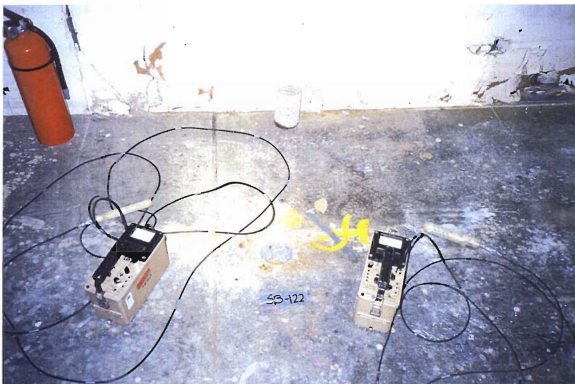
Soil boring SB-122 inside the former Gilbert Displays building. The radiation probes were used for downhole measurements
