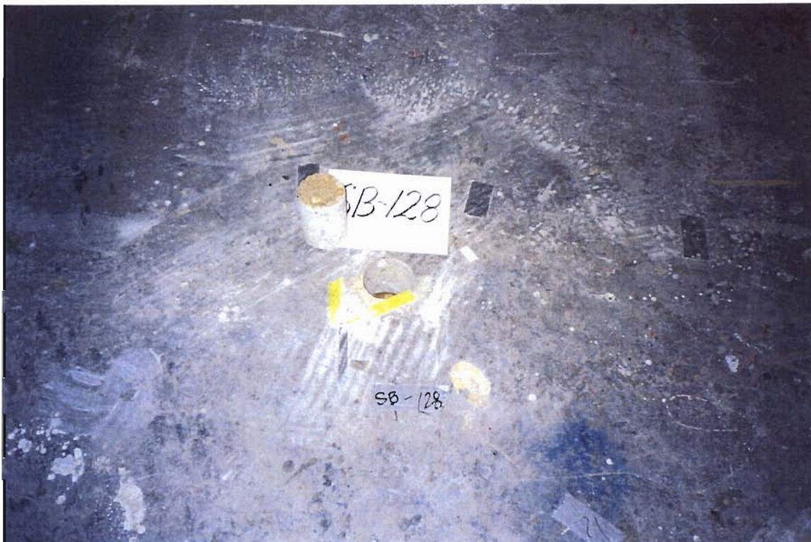
Soil boring SB-128, inside the former Gilbert Displays Building. This boring was placed to investigate surface levels of radiation.
