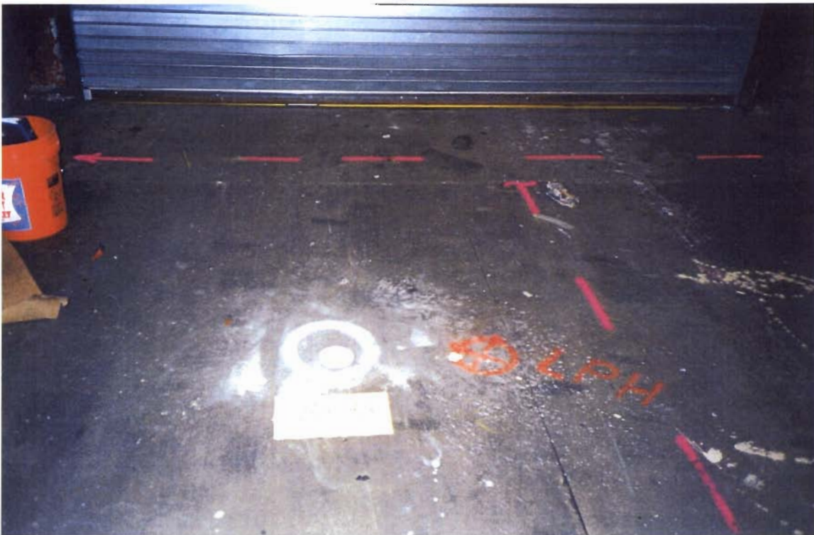
Soil boring SB-143 was placed inside the back door of Magazine Distributors to investigate an historic leaching pool.
