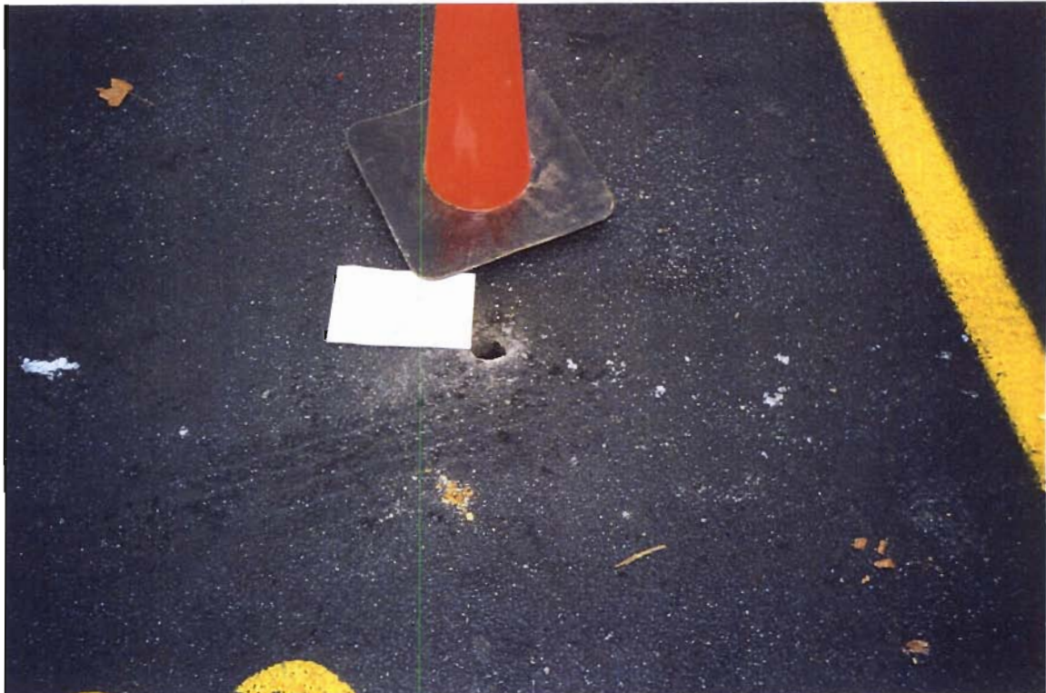
Soil boring SB-160 was used to delineate radioactivity near SB-003 at Air Techniques.
