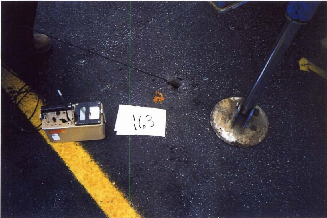
Soil boring SB-163 was used to delineate areas of surface radiation at Air Techniques.
