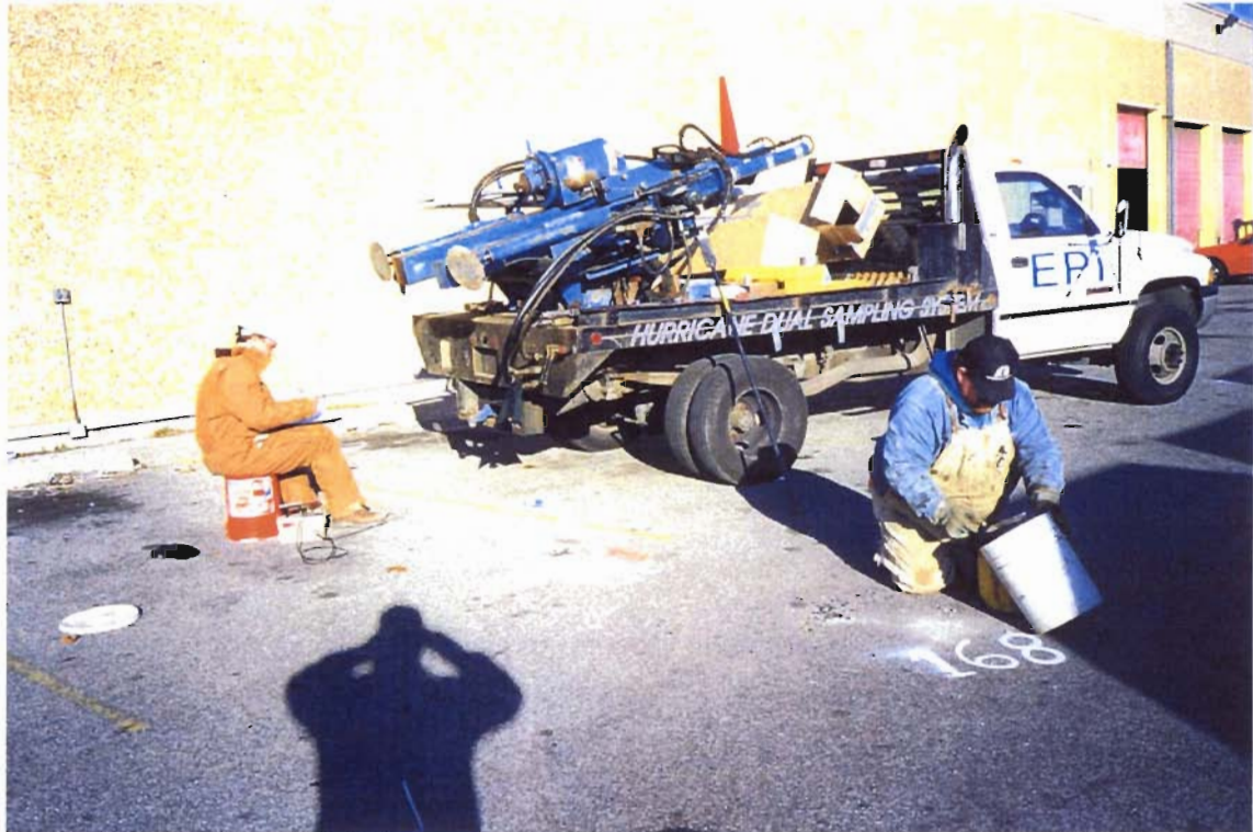
Soil borings SB-168 and SB-169 were used to delineate the extent of "green" material in SB-145.
