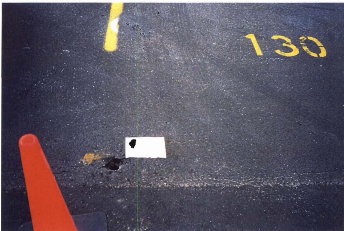
Soil boring SB-161 was used to delineate surface areas of radionuclides.
