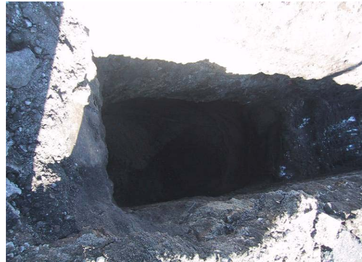
Photograph 12: Concrete slab at 5 to 7.5 feet bgs in TP-21, located at southern edge of former 3 million ft 3 gas holder footprint.
