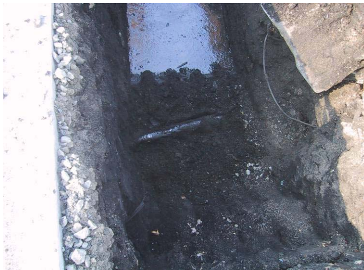
Photograph 23: Metal pipe and groundwater with sheen at 4 feet bgs in TP-33, located north of TP-32.
