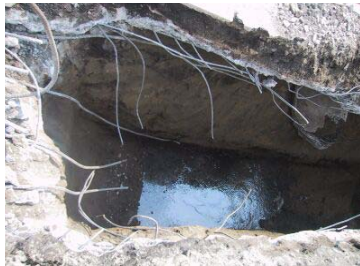
Photograph 24: Concrete pad with rebar and groundwater with sheen at 6 feet bgs in TP-34, located within footprint of former liquid petroleum process building.
