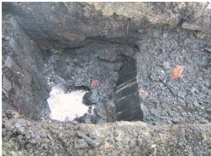
Photograph 17: Sheen on groundwater at 4 feet bgs in TP-25, located within footprint of former underground brick tar tank.
