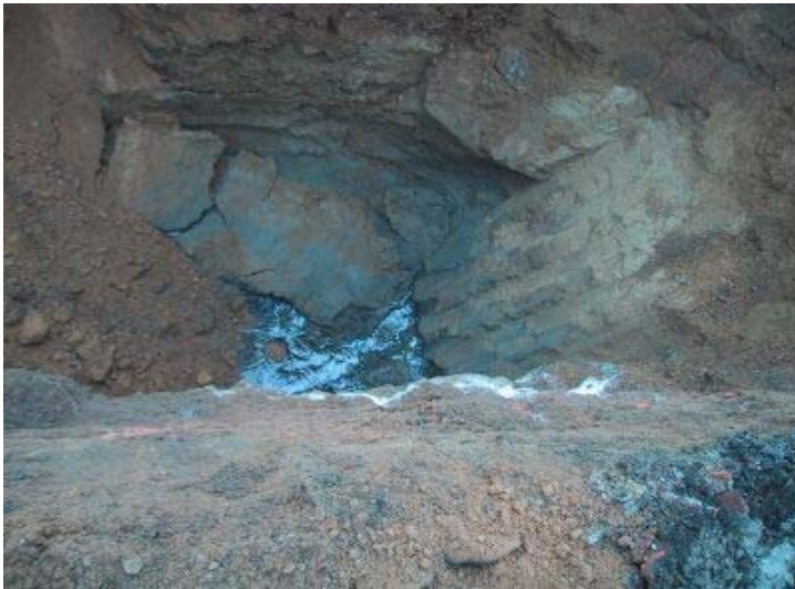
Photograph 15: NAPL at 8 to 10 feet bgs in TP-24, located within footprint of former generator house and adjacent to former underground brick tar tank.
