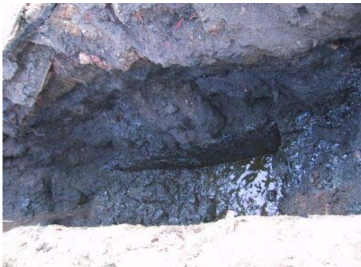
Photograph 21: Groundwater with sheen at 4 feet bgs in TP-31, located in southwestern portion of site, adjacent to Eastchester Creek.
