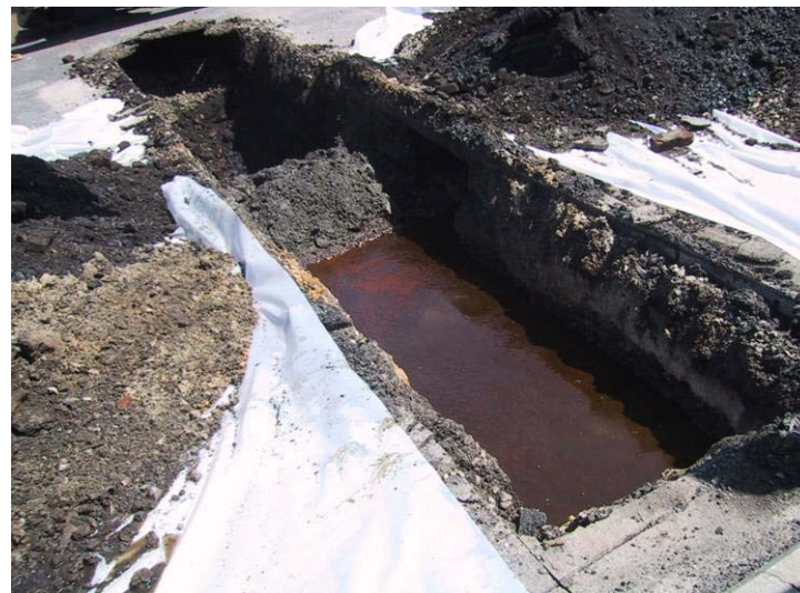
Photograph 22: Groundwater and NAPL at 2 feet bgs in TP-32, located in vicinity of former brick storage area.
