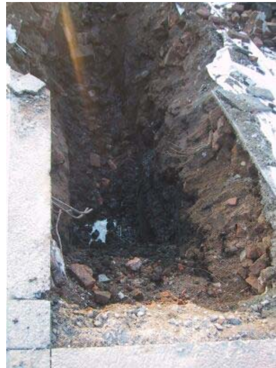
Photograph 20: NAPL and groundwater at 5 feet bgs in TP-29, located within footprint of former 100,000 gallon ammonia tank.
