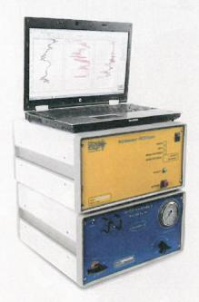
HPT produces a detailed hydrostratigraphic log
