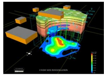
The end result of a UVOST boring is a high-density, non-subjective electronic data log (left) readily incorporated into accurate conceptual site models (top). Accurate source term models lead to knowledgeable decisions, accurate treatment and removal designs, and realistic cost estimates—saving time and money.
