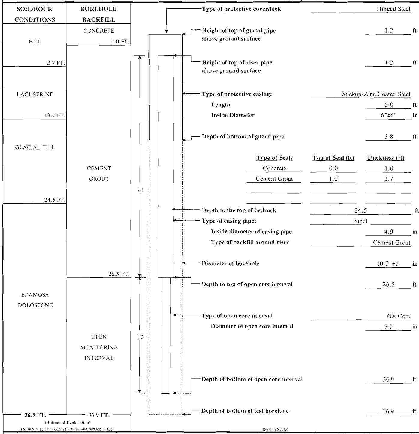
$$\text{Casing Length (L1)} + \text{Cored Interval (L2)} = \text{Pay length}$$
