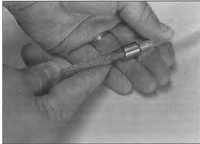
Attaching polyethylene tubing to the sampling implant.
