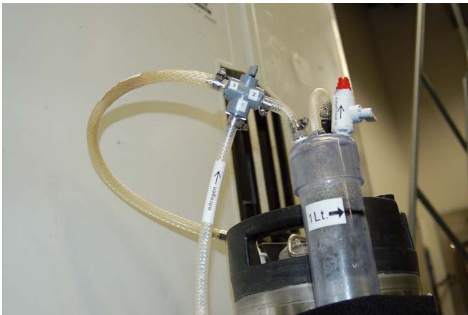
Measuring cylinder with attached three-way brass valve.
