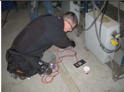
Photo 4 is a typical view of performance of diagnostic vacuum measurement utilizing a digital micro-manometer.
