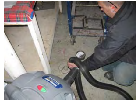
Photo 3 is a typical view of vacuum testing with a shop vac and magnahelic pressure gauge.
