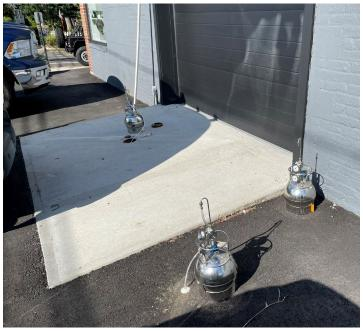
Photograph #1 - View of PP-3 located in concrete loading ramp. Also pictured: PP-2 and Outdoor Ambient Air.
