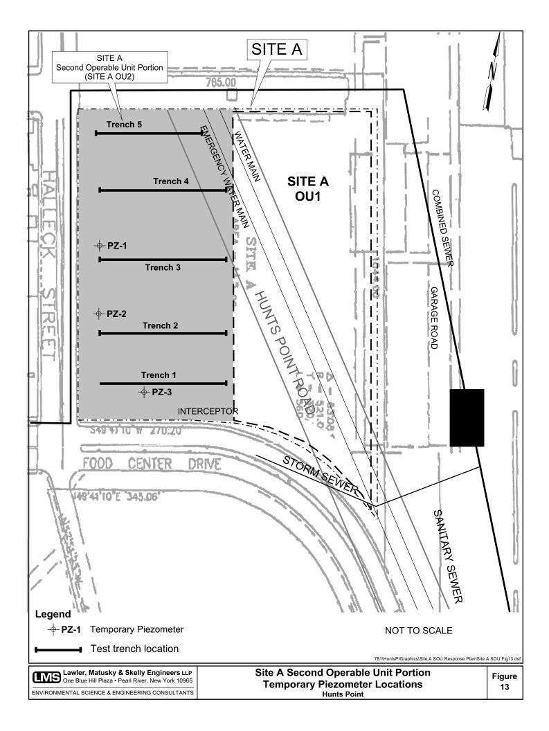
included as Attachment C. Sampling equipment was decontaminated between borings using cold wash techniques. Piezometers were installed to a depth of 5 ft below the water table and were constructed of 5 ft of 2-in inside diameter Schedule 40 PVC 0.010 slot screen and riser to grade. The piezometer was backfilled with #2 Morie sand to 2 ft above the top of the screen with a 2 ft bentonite seal, the remainder of the annulus of the boring was backfilled with cuttings from the boring to grade.
