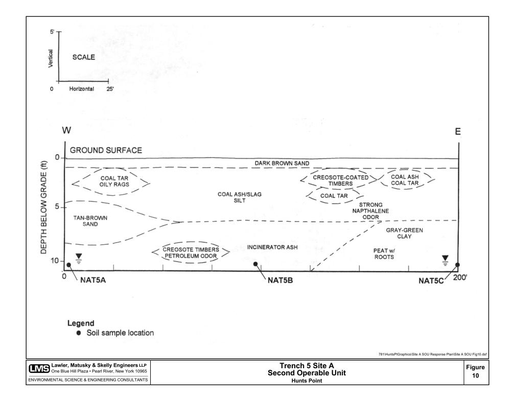
end of the trench. The middle layer of silt began to pinch out and a clay layer was present at 168 linear feet at a depth of 5 ft below grade. No other significant evidence of soil or groundwater contamination was present in this trench.
