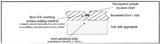
Schematic of Sub-Slab Vapor Probe to be Installed
