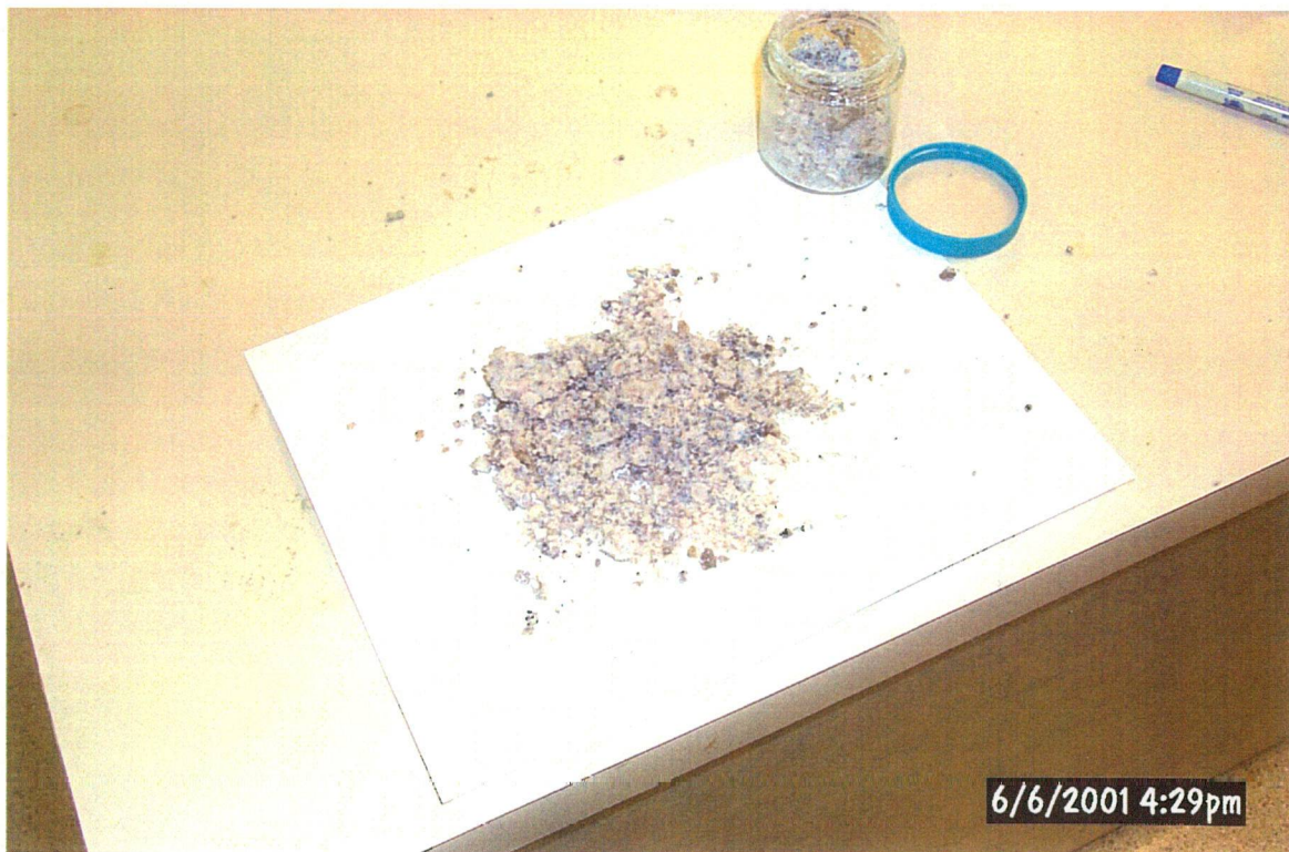
Photograph 2. Same soil sample as above from boring SB-213 after exposure to air.
