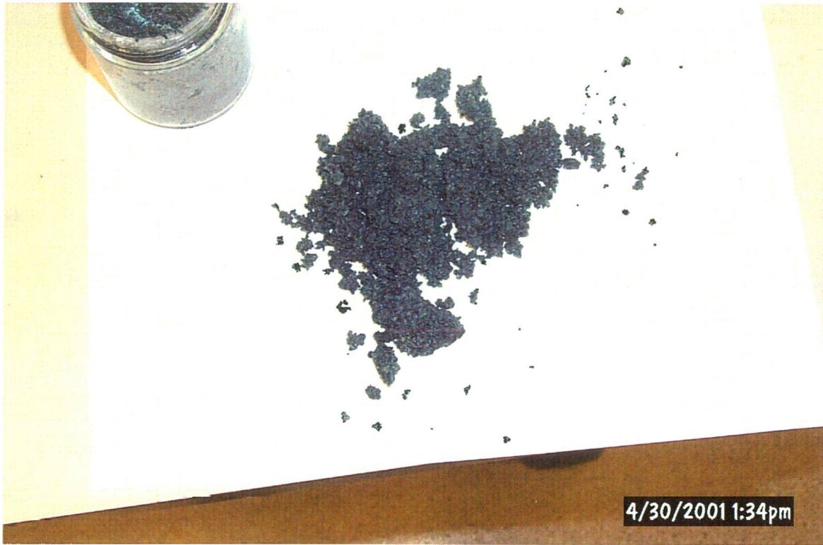
Photograph 1. Blue-green soil sample from boring SB-213.
