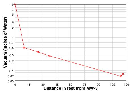
Based on the results of the pilot test, it was concluded that soil vapor extraction technology is a sufficient remedial alternative to mitigate residual soil and soil gas contamination at the Site. It was recommended that a soil vapor extraction system be designed and implemented to mitigate on-site sources of contamination.
