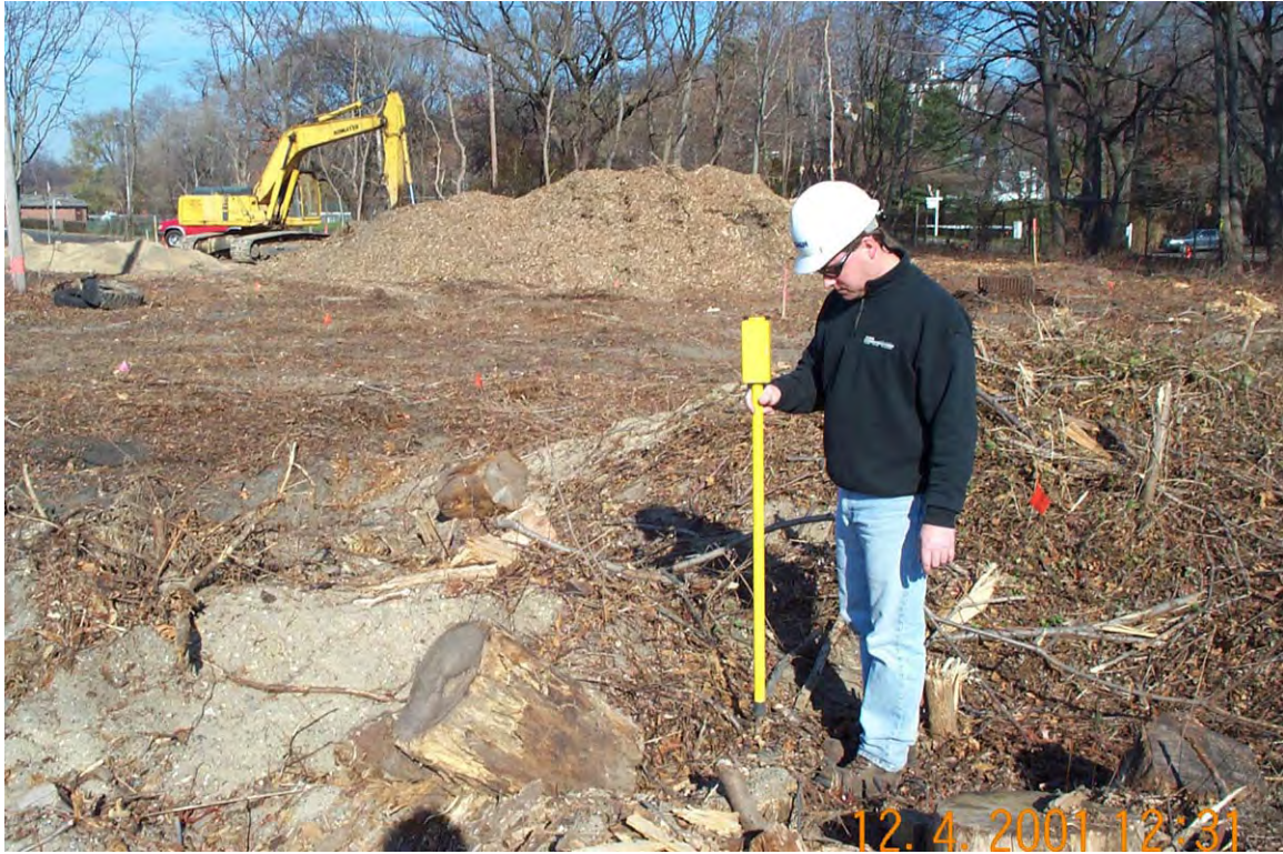
View looking northeast performing magnetometer survey in area 1B
