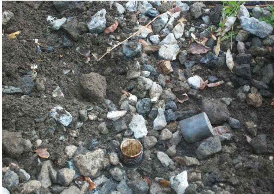
1. One-inch PVC pipe (MW-3), located in the northeastern corner of the Site, prior to decommissioning on December 3, 2013.
