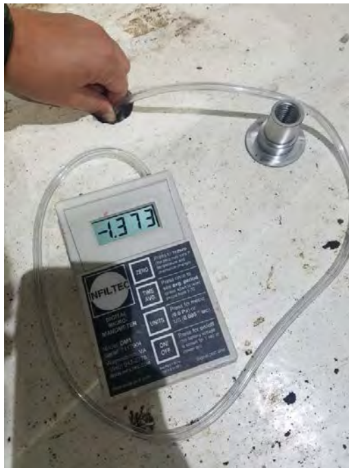
10. Sub-slab vacuum measurement
