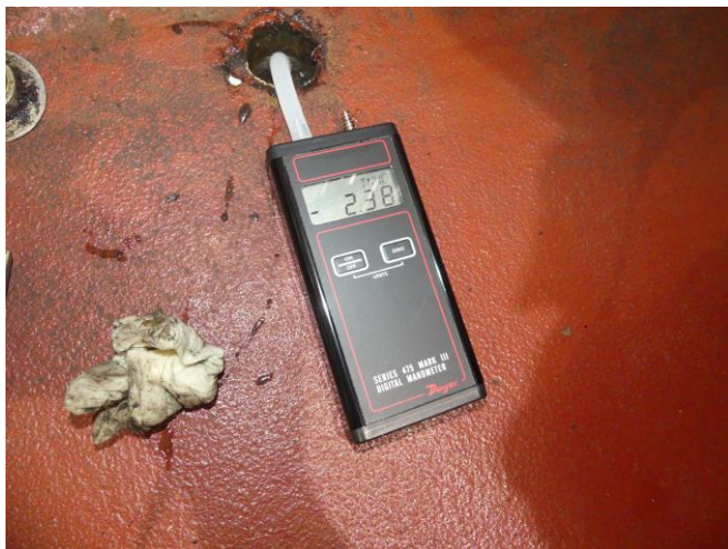
Sub-slab vacuum measurement of -2.38 IWC obtained after installation of new rooftop fan units. This measurement reflects significant improvement of vacuum from the previous measurement of -0.680 IWC taken on October 11, 2021.
