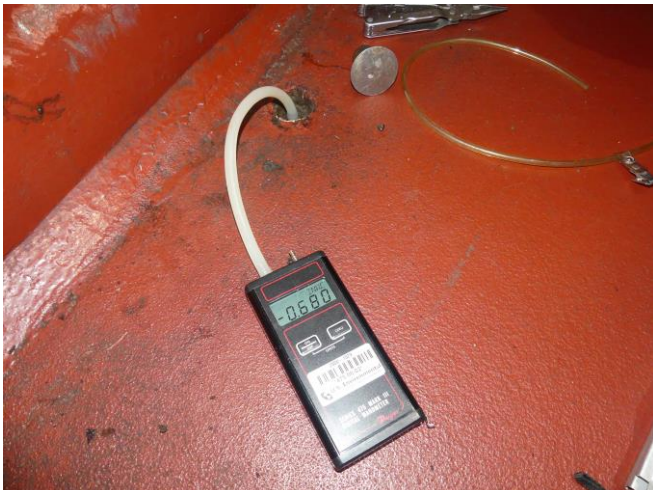
Sub-slab vacuum measurement of -0.680 IWC. Although lower than the previous reading from the 2018 PRR was -1.373 IWC, this vacuum indicates that the VES is operating sufficiently.
