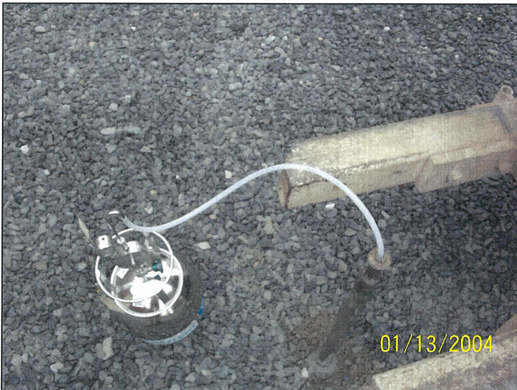
Photo 22. Overhead view of typical post-remediation soil vapor sample collection into Summa canister.
