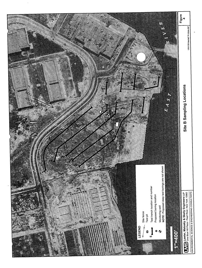
aboveground oil storage tanks (Figure 4). Trenches #3, #4, and #5 are located parallel to #2 and will extend through the areas where the greatest impacts were identified during the prior Phase II investigation. The downgradient northwest-southeast trench (#4) will be advanced through the area that contained the former propane storage tanks.
