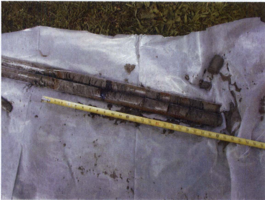
10. Example of distinct nature of subsurface NAPL impacts at depth (B-110).
