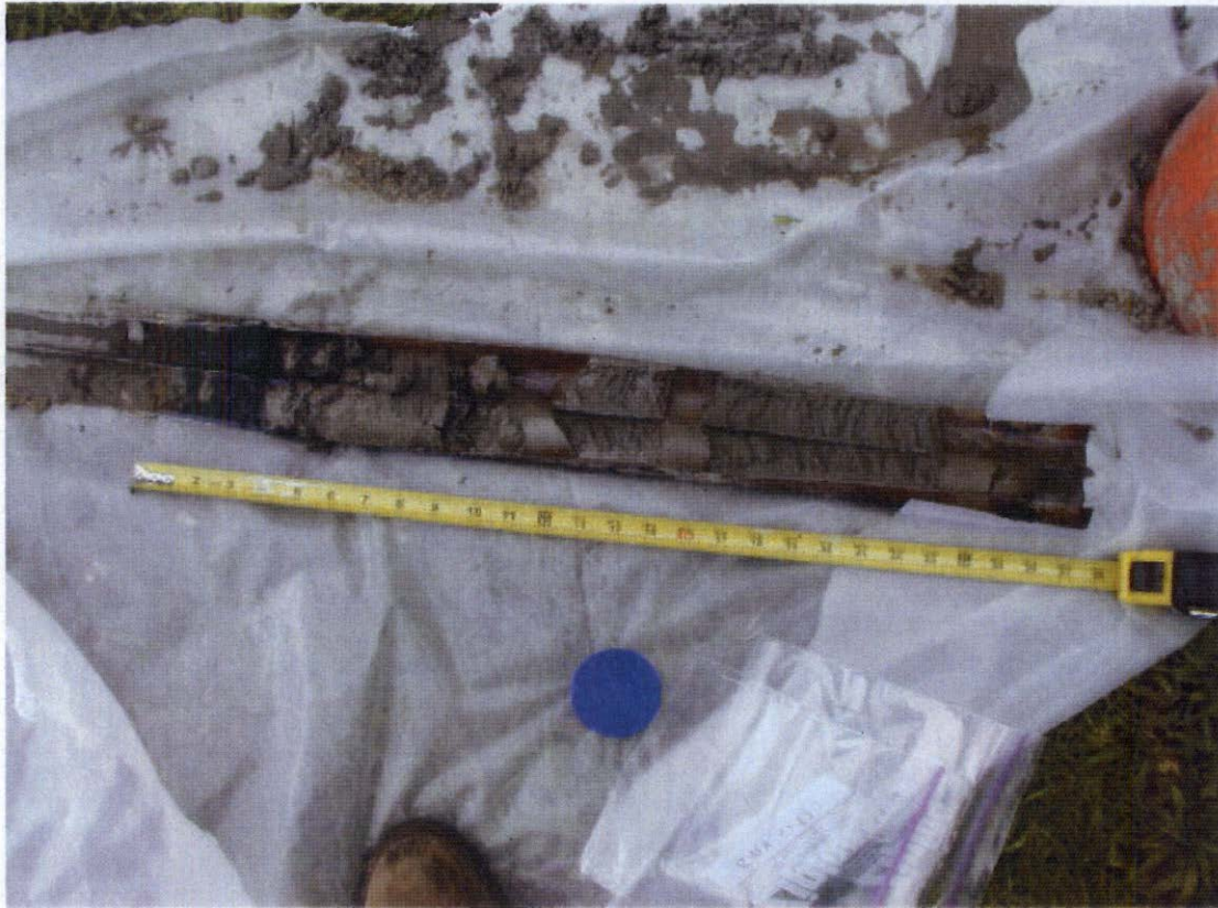
11. Example of distinct nature of subsurface NAPL impacts at depth (B-111).
