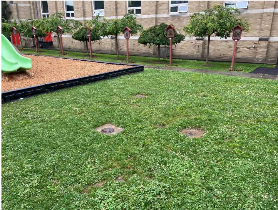
Photo 17: Monitoring Wells in St John's Courtyard (facing Southwest)
