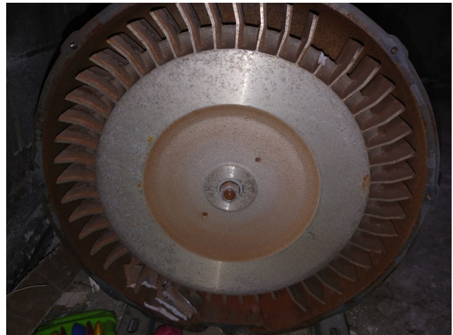
Photo 4: View of broken blades on blower of VES-1 during December 9, 2019 AWT site inspection.
