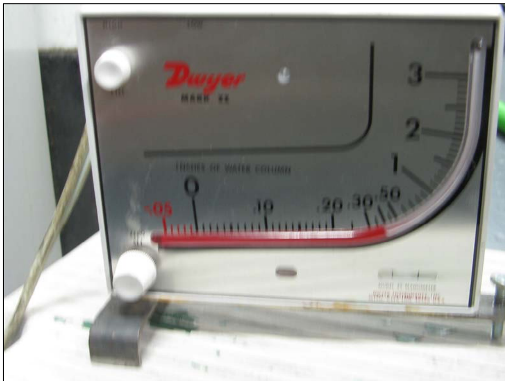
Photo 10. Vacuum gauge measuring -0.38 inches water at XP3 during pilot test.
