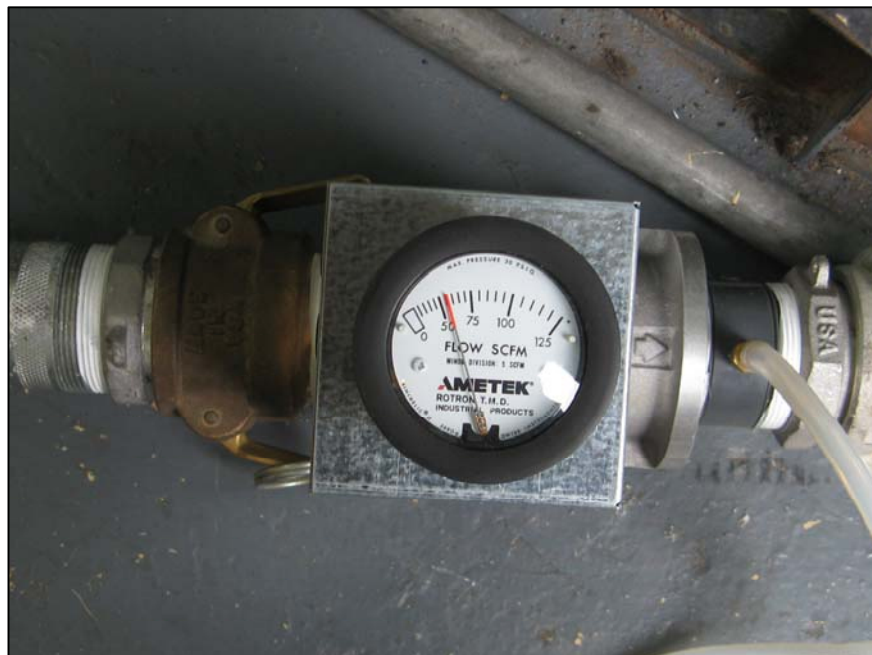
Photo 8. Air flow meter at 55 cfm for one hour pilot test monitoring flow from XP2 to shop vac.
