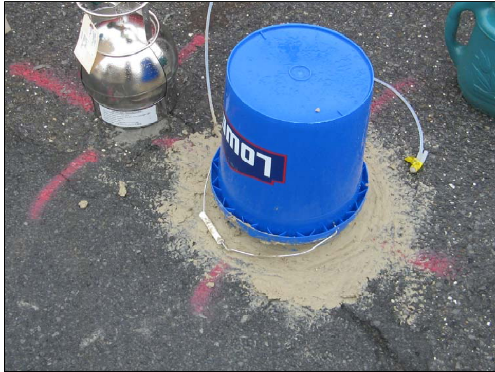
Photo 12. Setting up Summa sampling at SG25 with bentonite seal with canister & helium supply lines running under seal.
