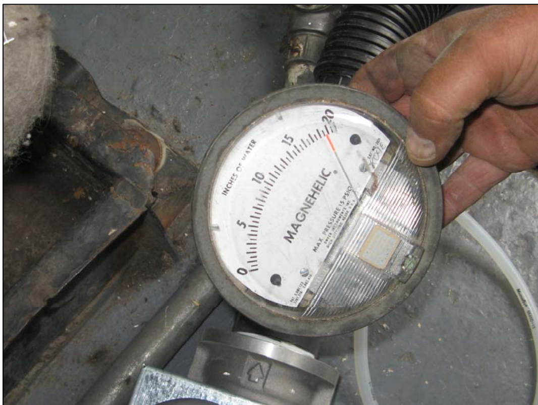
Photo 6. Vacuum gauge, blower on, no connection to XP2, -18.7 inches water.
