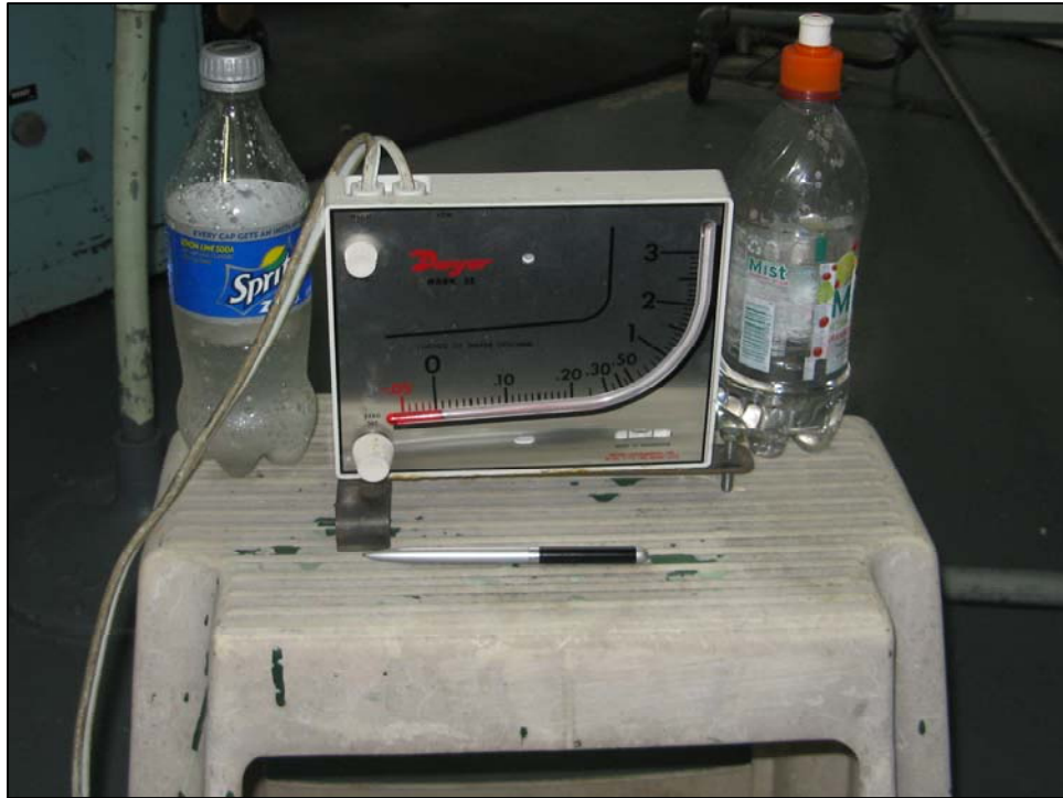
Photo 11. Vacuum gauge measuring -0.005 at temporary XP4 in far corner of building.
