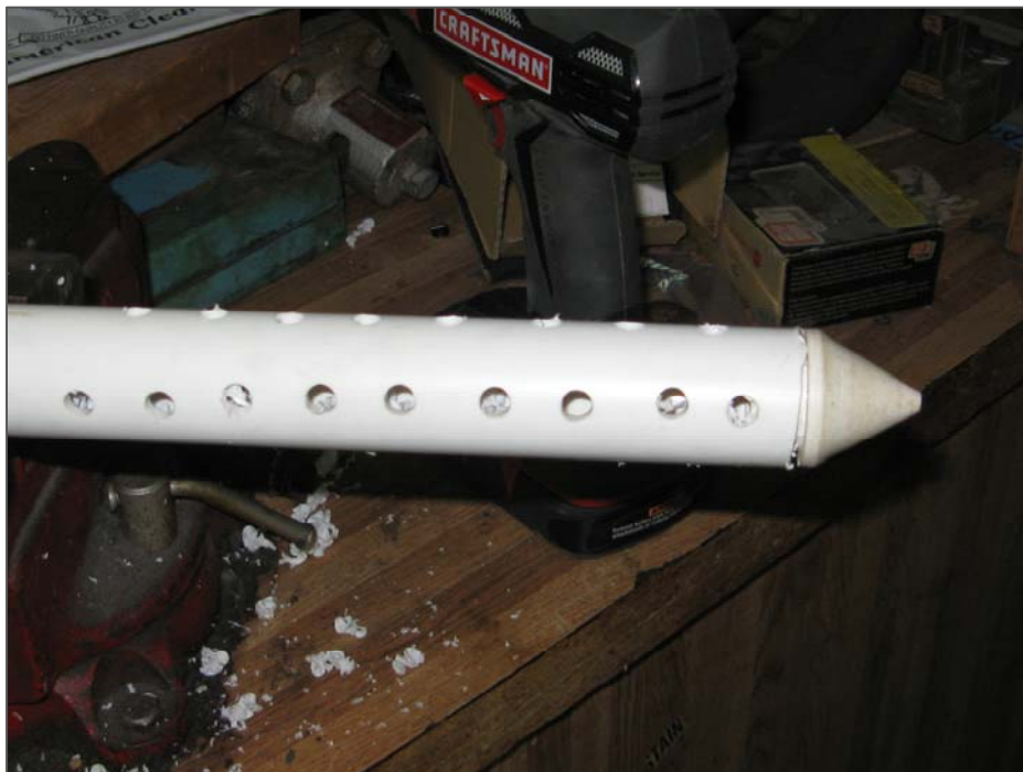
Photo 2. Vapor extraction "screen" prepared by drilling holes in 1-inch PVC to maximize air flow from sub-slab gravel.
