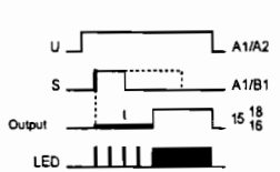
(J) On-delay (pulse controlled) (Min. Pulse AC 50ms – DC 30ms)
