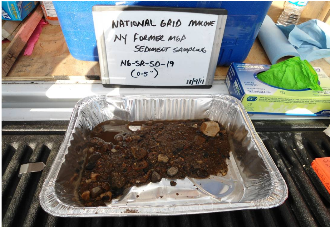
NG-SR-SD-19: Brown fine to coarse sand, little/some fine to coarse gravel. No impacts observed.
