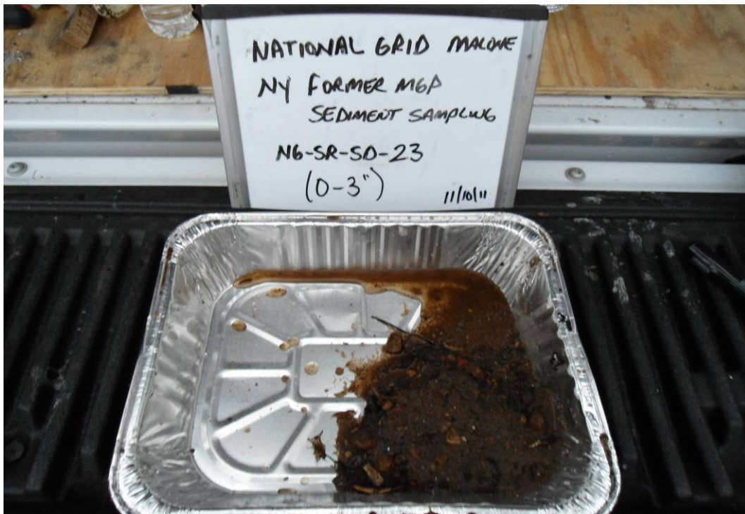
NG-SR-SD-23: Brown fine to coarse sand, little fine to medium gravel, trace organics (vegetation/twigs). No impacts observed.
