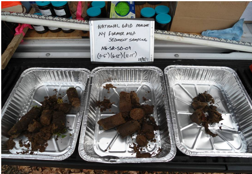
NG-SR-SD-09: (0 – 6") Dark brown fine sand, trace silt, trace organics (roots). (6 – 12") Same as above (SAA). (12 – 14") SAA, trace wood. No impacts observed in samples.
