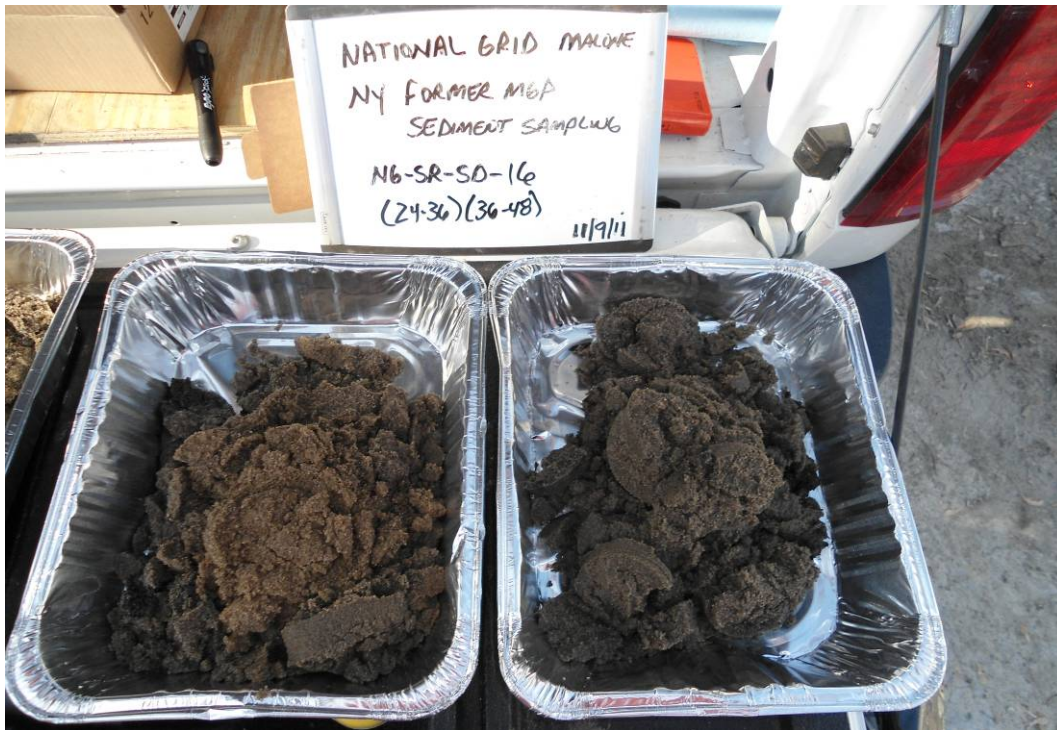
NG-SR-SD-16 (Continued): (24 – 36”) Brown fine to medium sand, trace wood. (36 – 48”) SAA. No impacts observed in samples.
