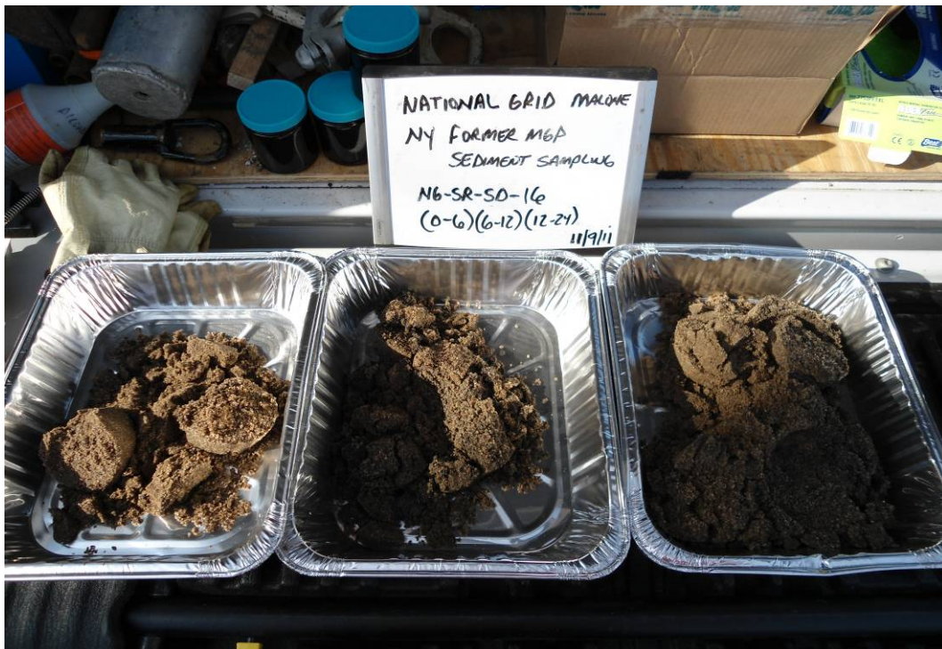
NG-SR-SD-16: (0 – 6”) Brown fine to medium sand, trace organics (vegetation). (6 – 12”) SAA. (12 – 24”) Brown fine to medium sand. No impacts observed in samples.
