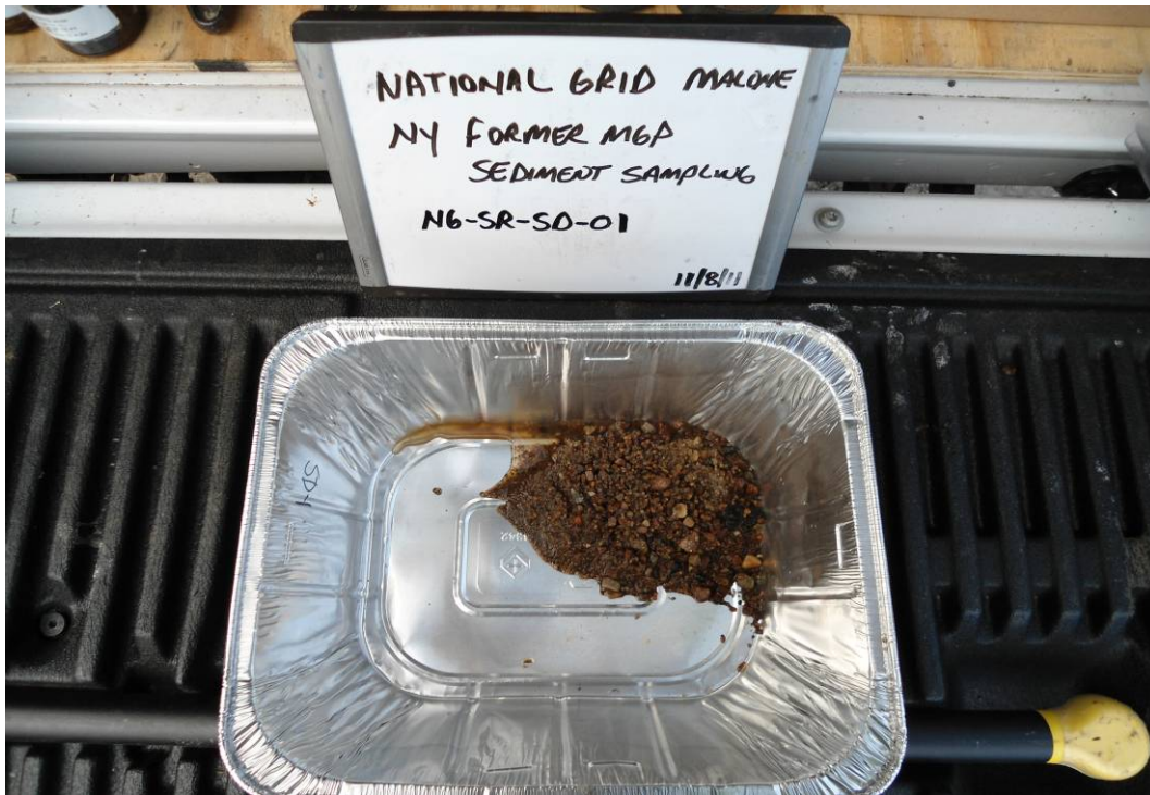
NG-SR-SD-01: Gray brown fine to coarse sand, little fine gravel. No impacts were observed.
