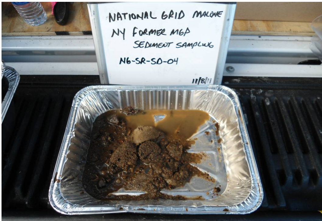
NG-SR-SD-04: Gray brown fine to medium sand, trace coarse sand, trace fine to coarse gravel. No impacts observed.
