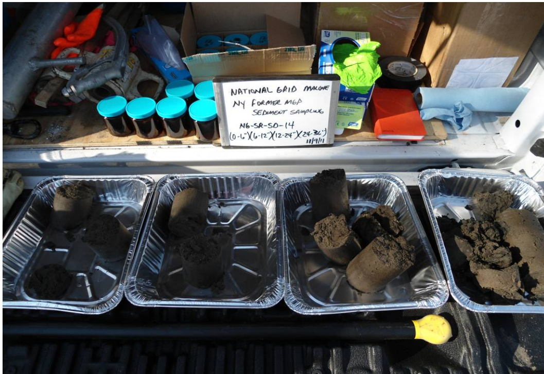
NG-SR-SD-14: (0 – 6") Brown fine sand, trace organics (roots). (6 – 12") SAA. (12 – 24") SAA, trace silt. (24 – 36") SAA. No impacts observed in samples.
