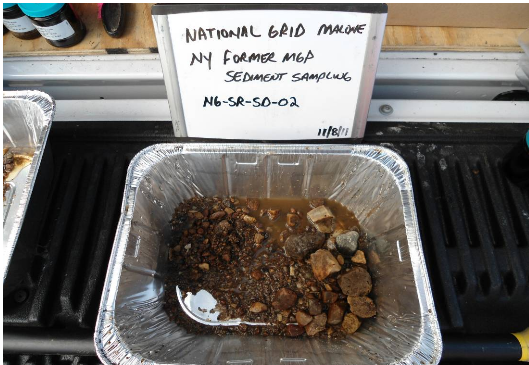
NG-SR-SD-02: Gray brown fine to coarse sand, little/some fine to coarse gravel. No impacts observed.
