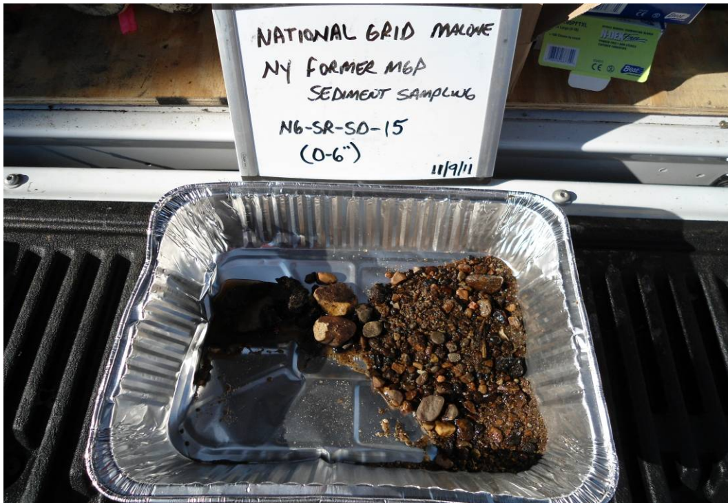
NG-SR-SD-15: Brown fine to coarse sand, little fine to coarse gravel. No impacts observed.
