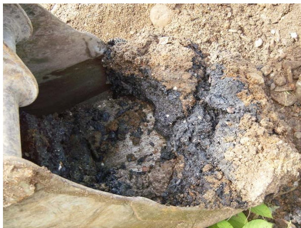
Figure 3-4 Tar encountered in CTP-2 on Pritchard Property
