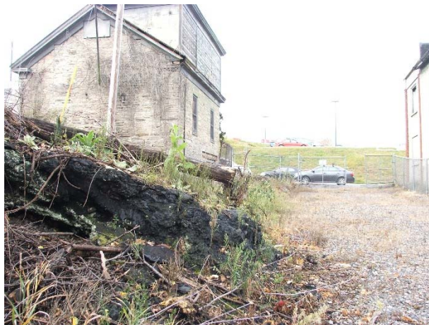
Figure 3-2 Solid tar observed on ground surface of site, looking toward Amsden Street, former MGP building on left
