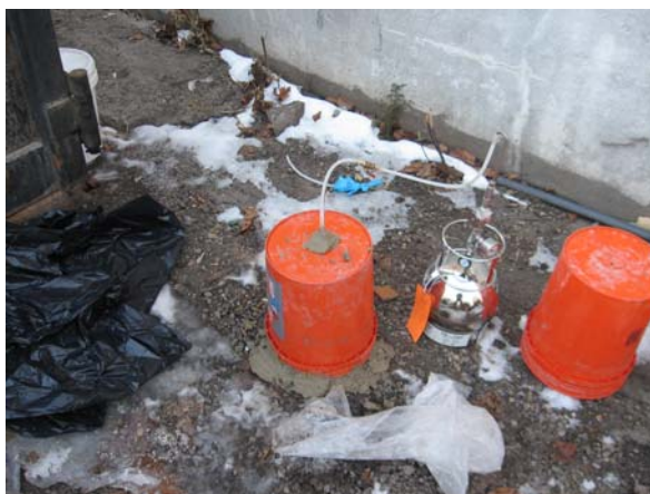
Figure 2.2: Typical Setup for Soil Vapor Sampling, SV-1 (St. Lawrence Foods) shown
