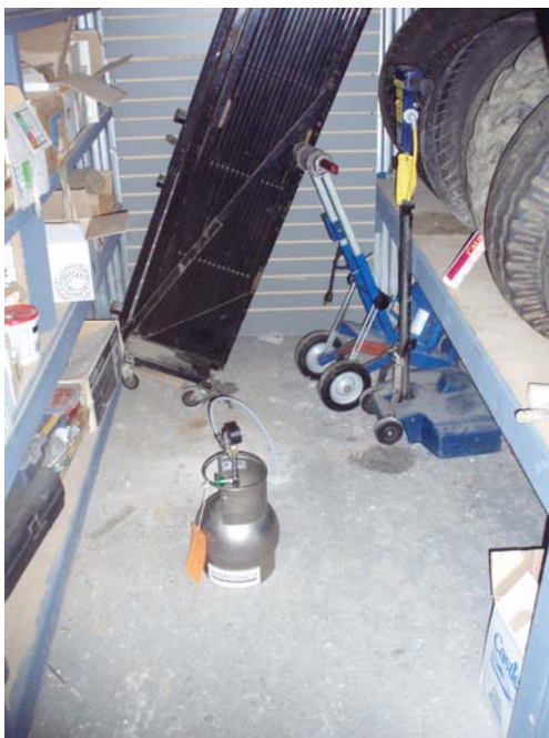
Photograph #15 – Sub-slab vapor sampling performed at Taylor Rental on March 18, 2008.
