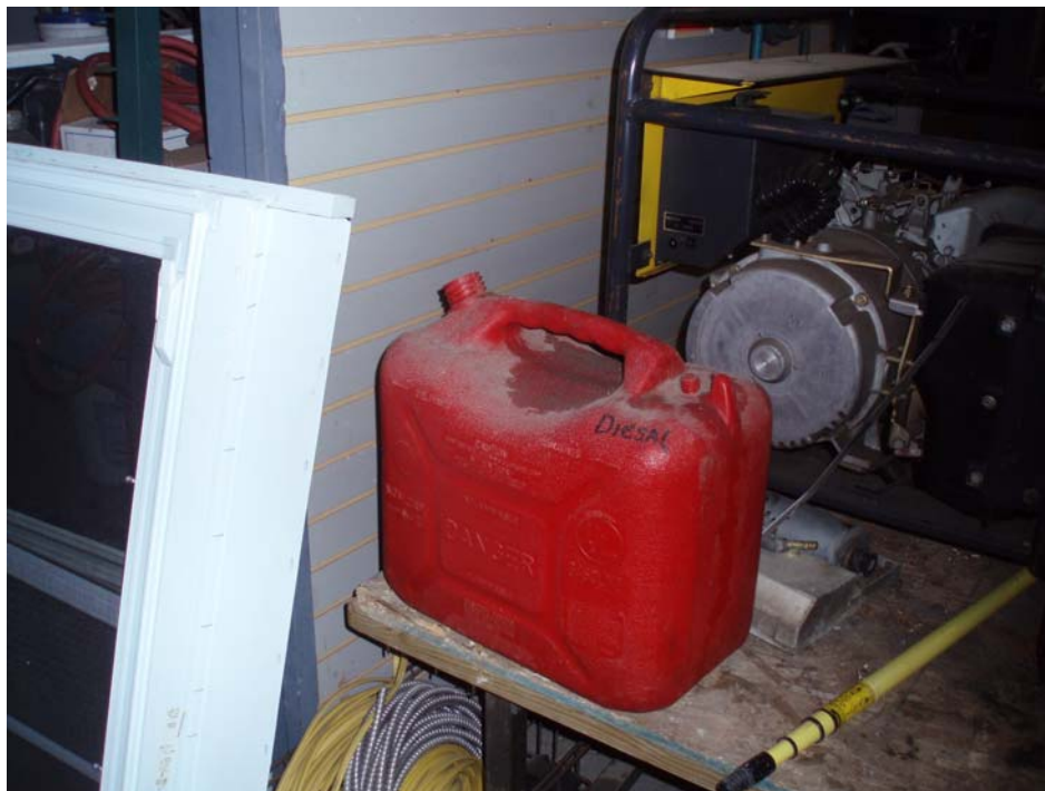
Photograph #7 – View of open container of fuel. Reading of area surrounding container was 73 ppm using photoionization detector (PID).
