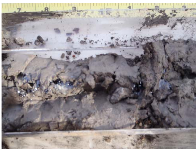
2 mm vertical lens of black NAPL in boring B-517(13) between 11.3 and 12.3 feet bgs.
