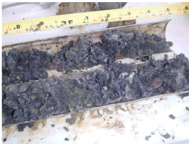
Thin (1 mm), sticky tar stringers in boring B-519(13) between 20.1 and 21.2 feet bgs.
