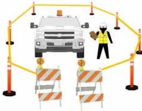
Intermediate Term (1-8 Hours) Channelizing Cones, Caution Tape and Type II Barricades
