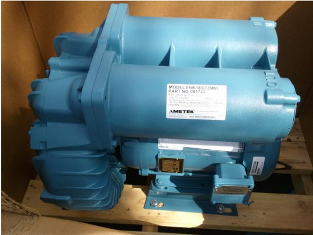
Photo 3: View of spare SSDS fan unit delivered on March 12, 2012.
