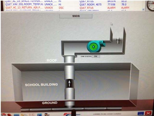
Photo 1: View of the BMS indicating SSDS operation.
