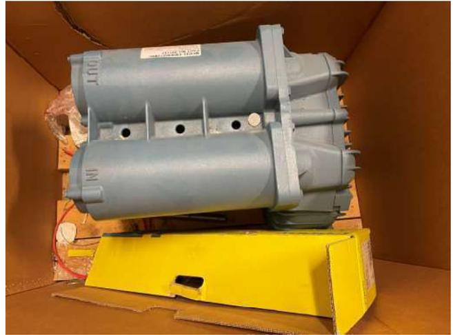
Photo 2: View of the spare SSDS motor unit.
