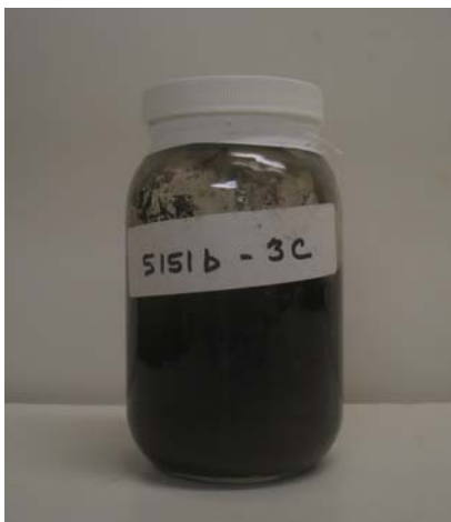
Photograph 1: Laboratory set up of the batch jar. 500 mL jar with 300 g of unsaturated soil.
