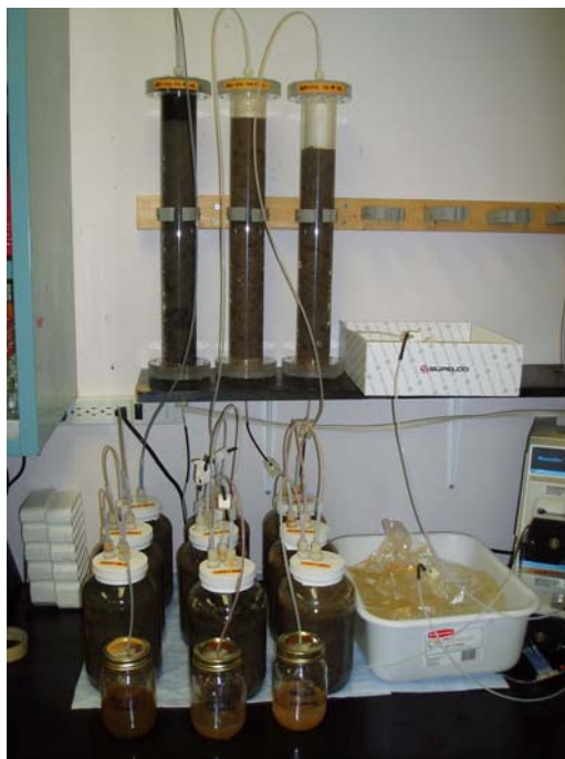
Photograph 2. Laboratory set up of the columns. Each system consists of a column followed by three soil microcosms. Systems 1-3 (left to right).
