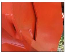
The overlapping side plates increase the cross-sectional area of the sides of the bucket, enclosing the material inside of the bucket with no where to go.
