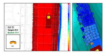
Projects requiring uniform removal over a specified area can be difficult for some dredging systems. (Ex. the bottom is constantly sloping and the specifications call for 1 ft of material to be removed throughout.) ClamVision has a separate mode specifically for these situations. In this mode, color is no longer directly tied to depth, but is tied to the "distance to completion."
