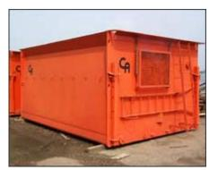
This can either be a stand alone wash tank manufactured by Cable Arm, or some other piece of equipment converted to a wash tank.
