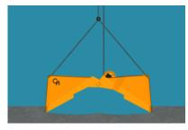
As the clamshell closes, the sides draw together and the pivot point lifts, leaving a large rectangular footprint that is very close to level.
