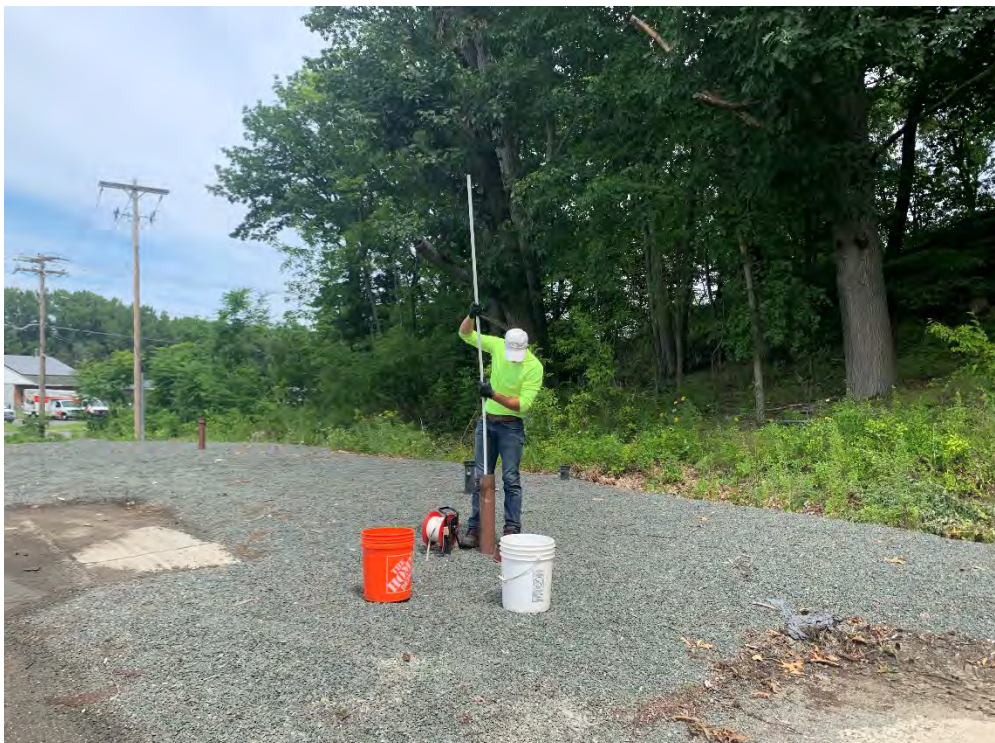
Photo 18: Attempting to dislodge formerly deployed PDB in MW-2 (facing northeast).
