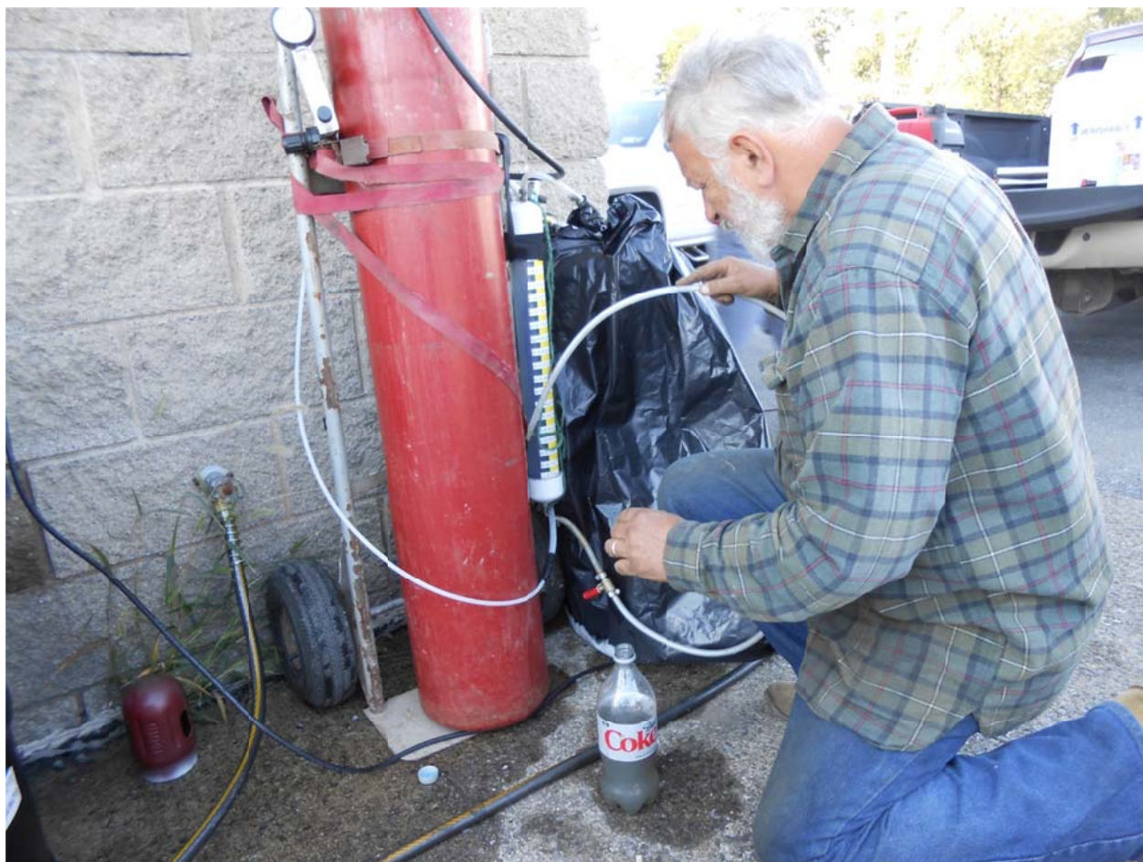
P42. Preparing to 0.75 liters of inoculum into the calibrated 1 liter coke bottle. The calibrated sight glass to the right of the red nitrogen tank shows the volume of inoculum pumped out into the bottle using the nitrogen pressure from the tank. October 8, 2015
