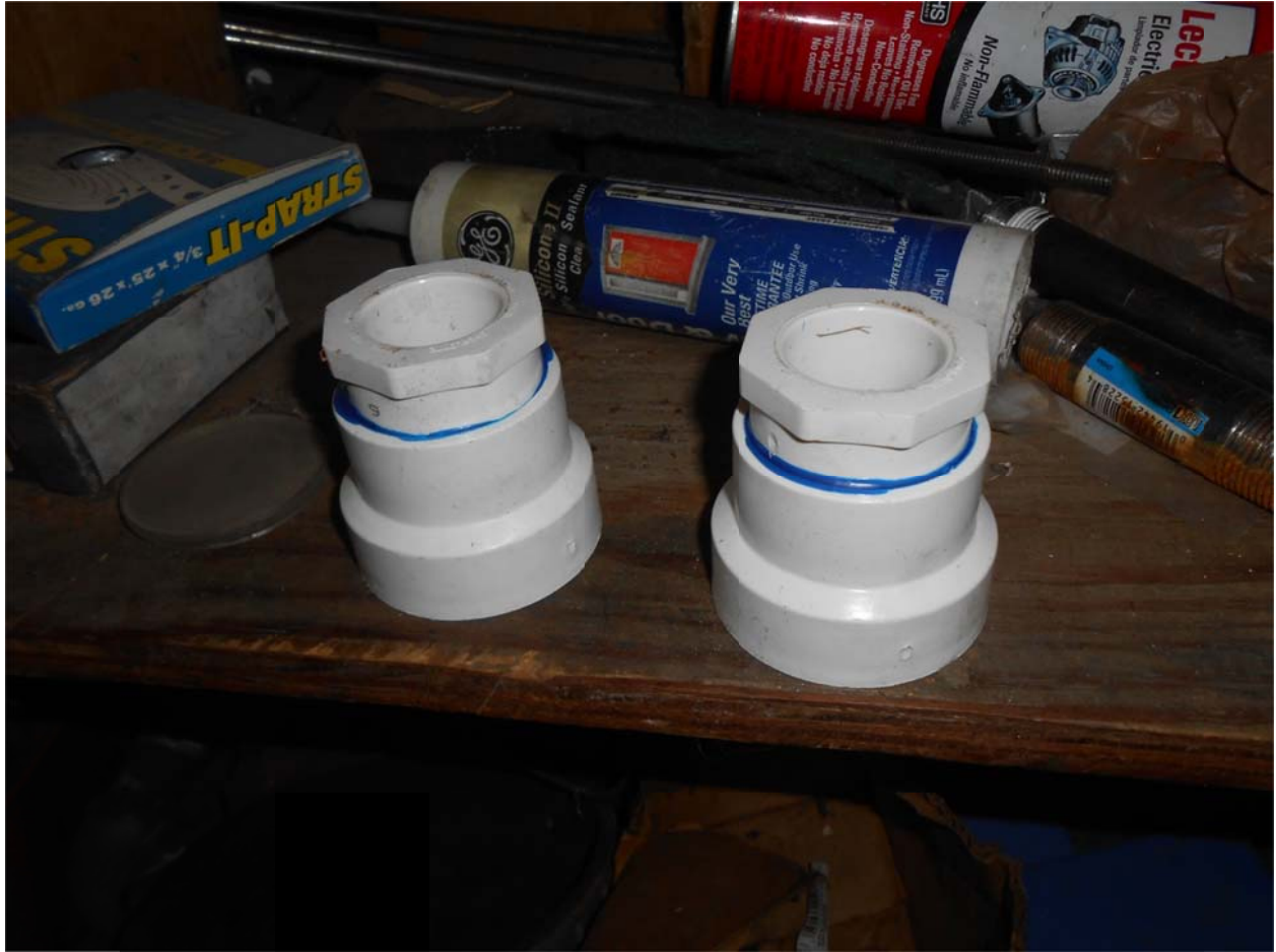
P21. Adapters for top of 2-inch PVC shaft above the roof to accommodate the 4-inch Stainless Turbines. For strength a glue had to be used to attach the components. 4/10/15
