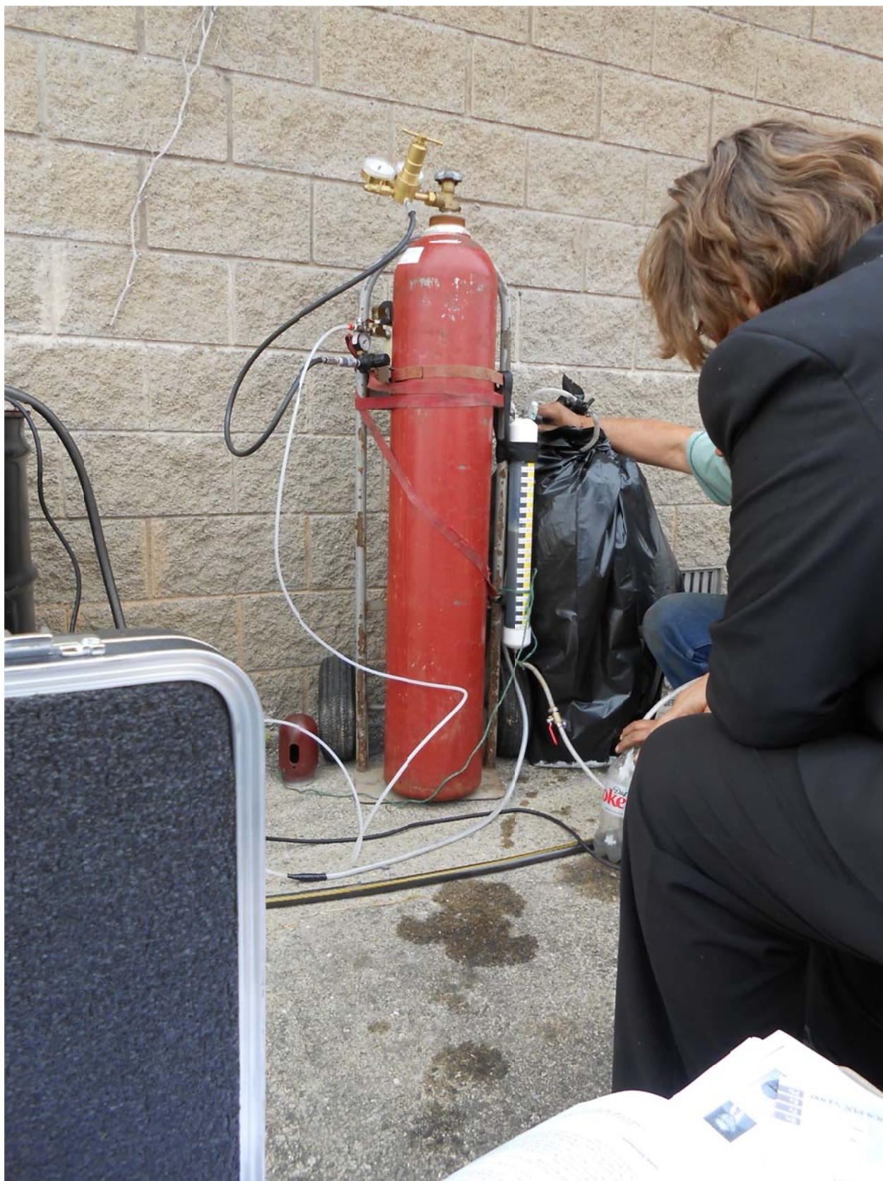
P40. The inoculum is stored in the keg which is inside the black plastic bag. Dry ice is used to maintain the temperature at 2-4°C inside the bag or inside the cooler, where ever the keg is stored. October 7, 2015
