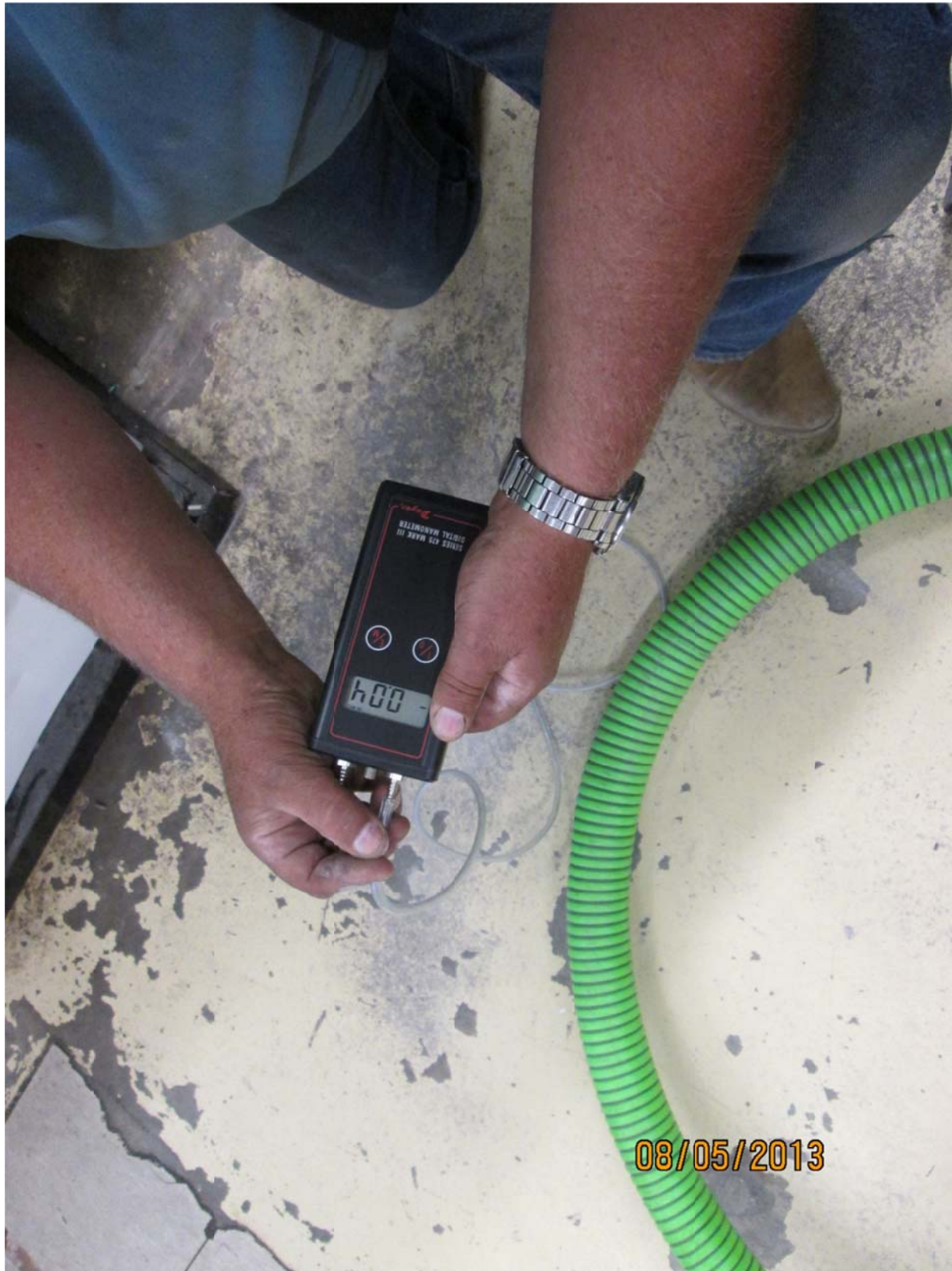
XP16. Vacuum of -0.04 inches of water measured at VP2 105 inches from XP3 where vacuum was applied with blower. 8/5/13
