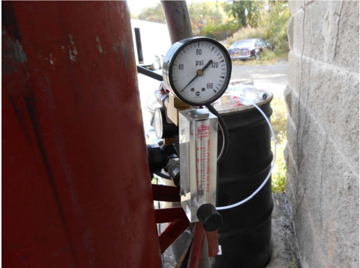
P37. Nitrogen in the red tank sparging into water in the 55-gallon black drum to deoxygenate the water to use with injection of the inoculum. Pressure meter (in PSI) and flow meter (in SCFM) used to control rate of sparging are shown to the right of the tank. October 7, 2015
