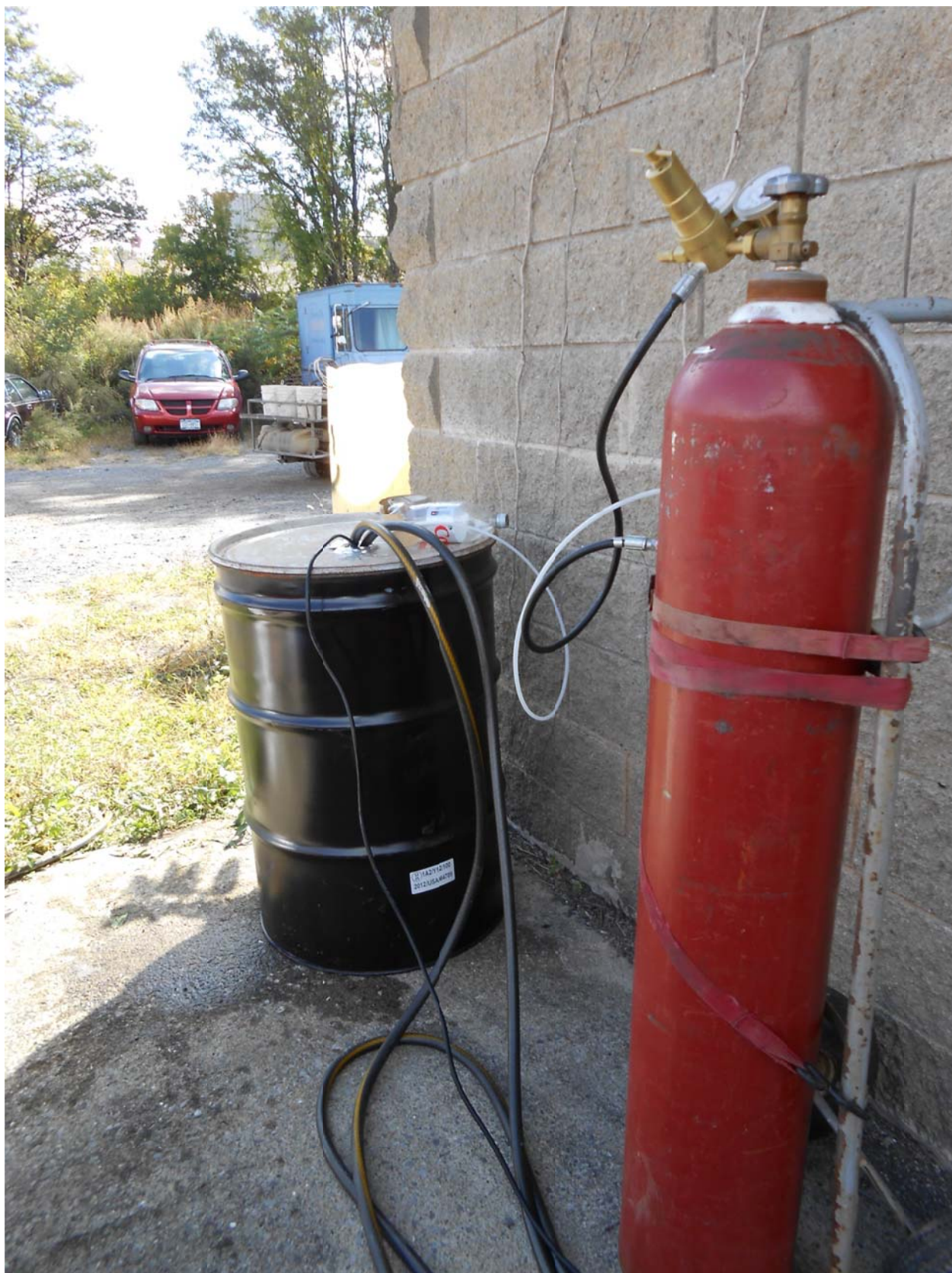
P38. Red nitrogen tank and black deoxidizing drum. From the outdoor spigot, the water supply hose goes into the drum. A submersible pump in the tank pumps the water through the output hose to the GS2000 pump hopper. October 7, 2015
