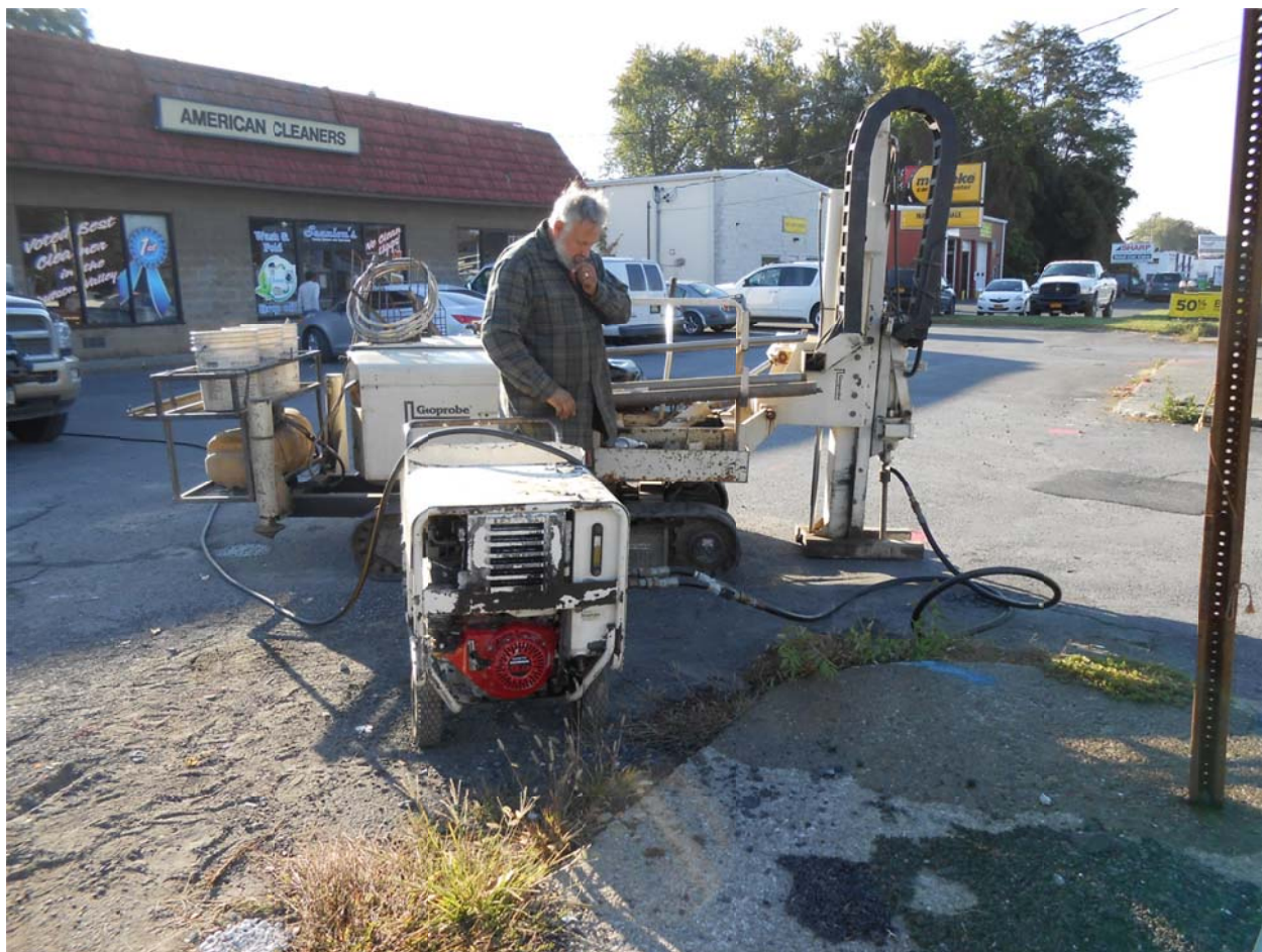
P45. GS2000 pump in the foreground showing the input hose from the pump to the Geoprobe drill rods. October 8, 2015
