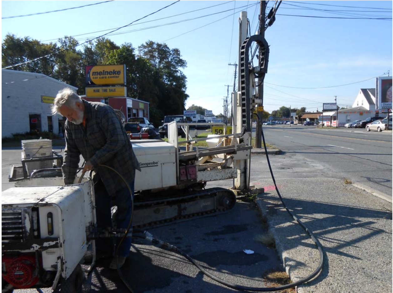
P41. Pumping the measured amount of deoxygenated water into the hopper of the GS2000 high pressure pump for mixture with inoculum and injection into subsurface injection point with the Geoprobe. October 8, 2015
