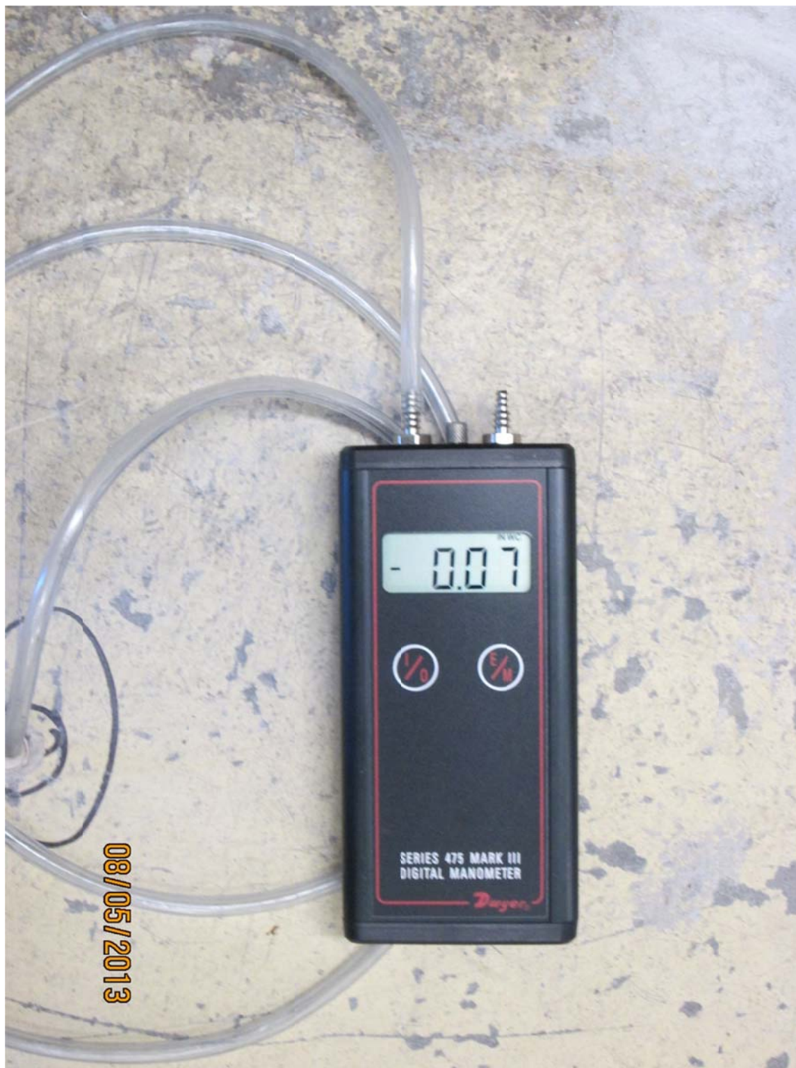
P12. Manometer measuring a vacuum of -0.07 inches of water at VP1 located 5 feet southwest of XP2 while vacuum is applied to XP2 using a 1 horsepower Fuji Blower. 8/5/13
