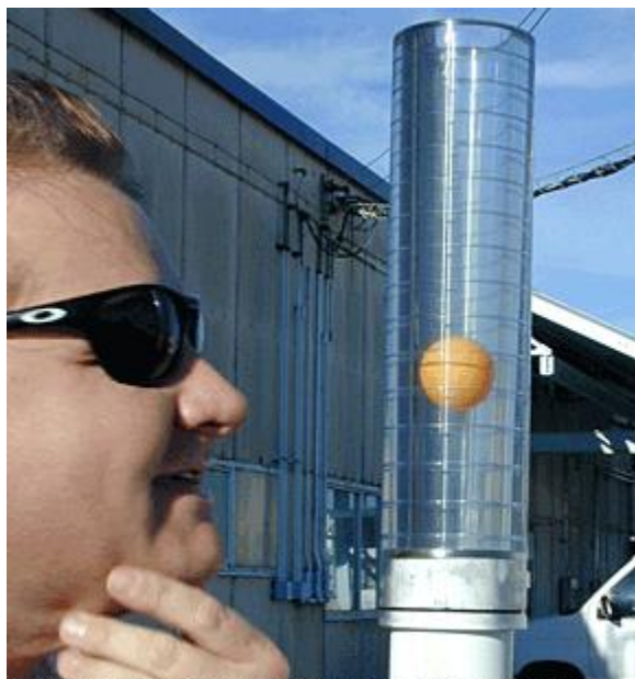
Dennis Jackson of SRS examines natural flow out of a well with the help of a BaroBall.
