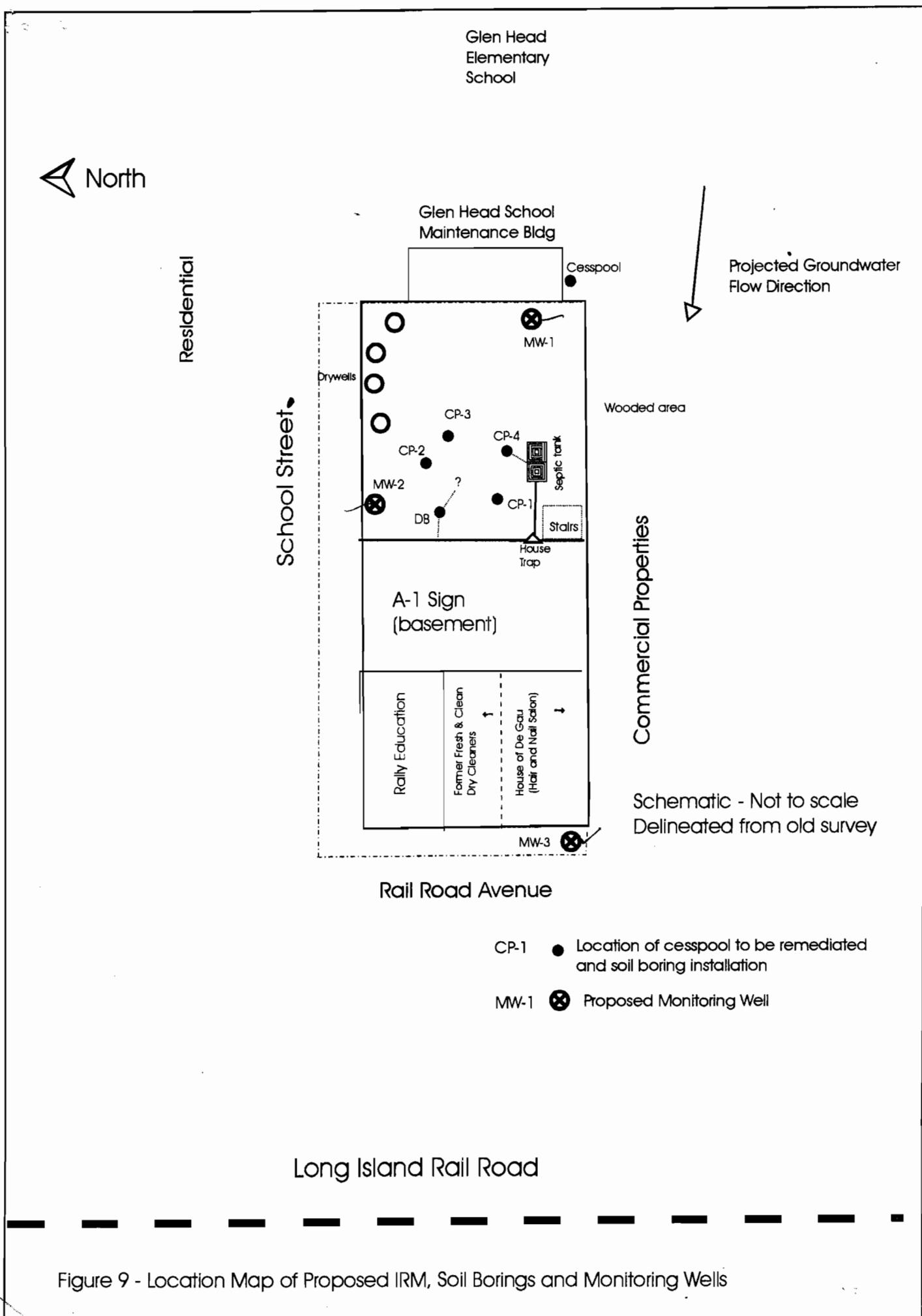
Figure 9 - Location Map of Proposed IRM, Soil Borings and Monitoring Wells
