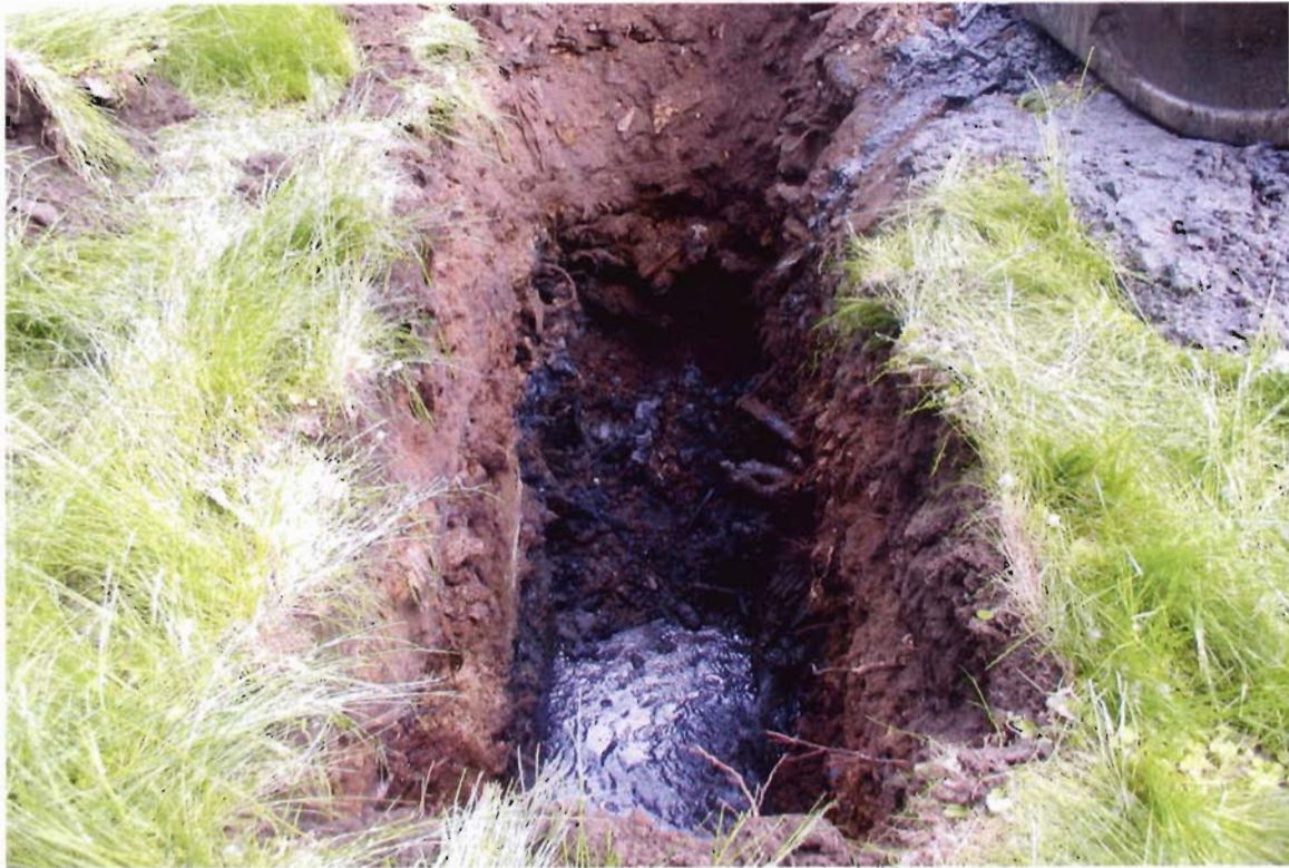
Photograph 15. Stratigraphy of material and groundwater within ZR-TP-08
