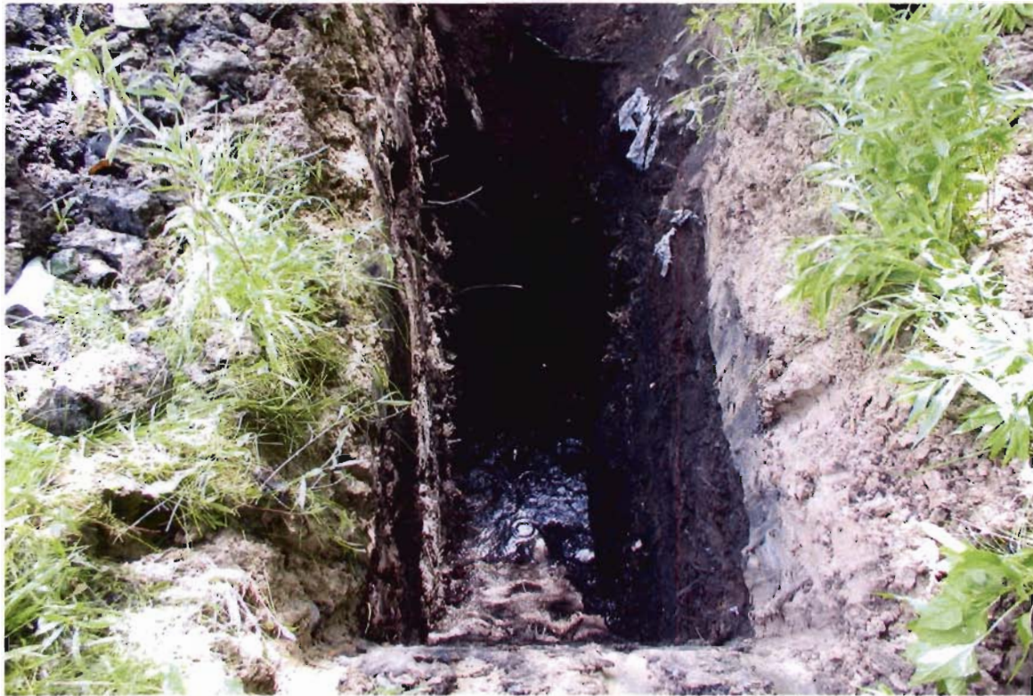
Photograph 7. Stratigraphy of material and groundwater within ZR-TP-11
