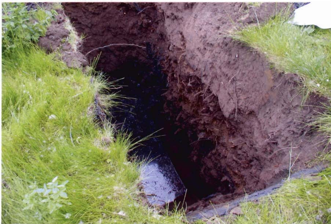
Photograph 11. Stratigraphy of material and groundwater within ZR-TP-09
