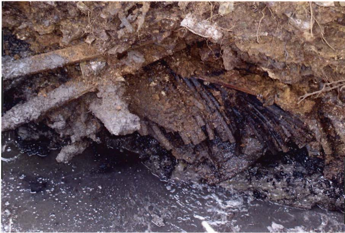
Photograph 17. Material and perched groundwater within the trench ZR-TP-08
