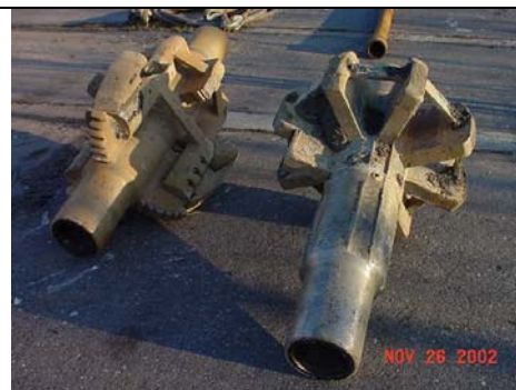
Photo 8. Stripped 44 inch Reamer
