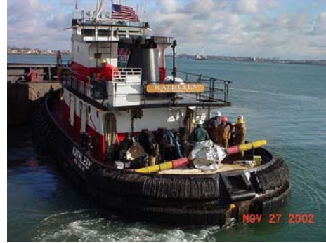
Photo 10. Boating Reamer to Barge
