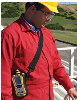
MultiRAE used for worker exposure monitoring at an oil refinery
