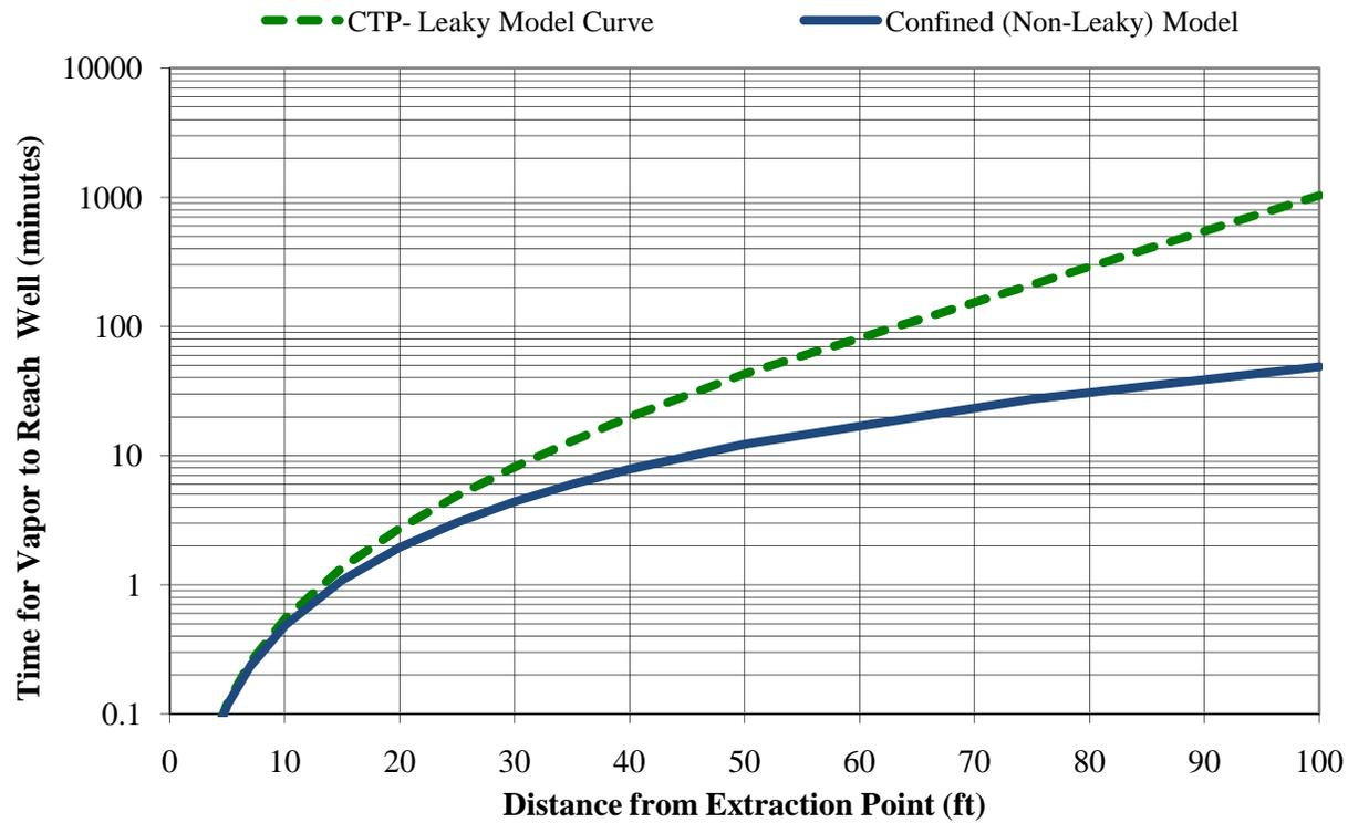
Note: Travel time of 1 day (1440 minutes) extends to a radial distance of 95 feet from extraction point
