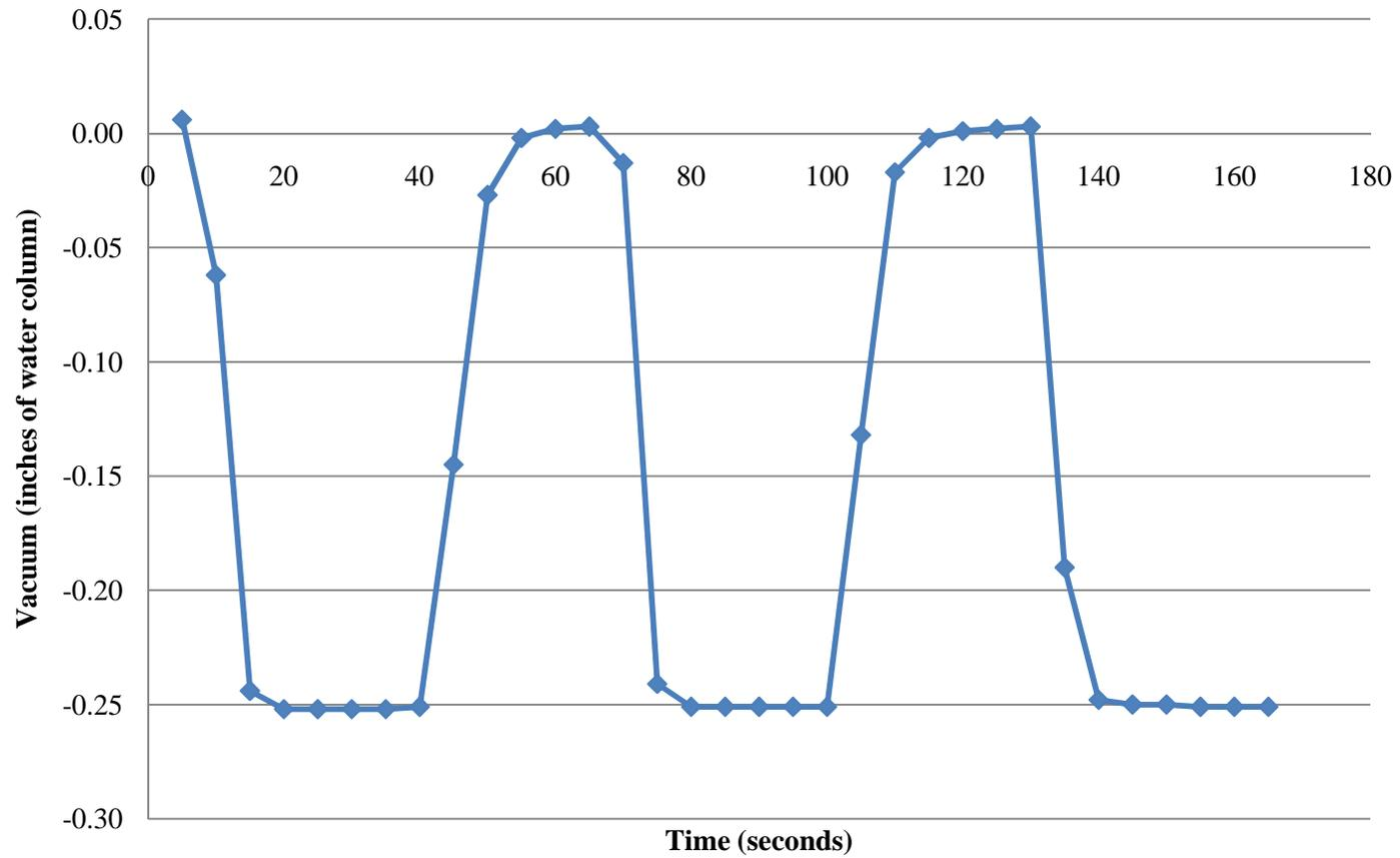
**Figure 2: Graphical Output of Hantush-Jacob Model Fit to Transient Vacuum Versus Time Data**
