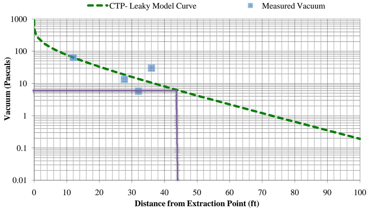
**Figure 4: Comparison Between Sub-slab Soil Gas Velocity Calculated From Leaky Aquifer Model and Non-Leaky Model**
