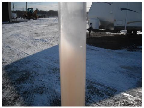
Photo No. 8. View of purge water in MW-13 prior to sampling. Water is turbid but does not reveal purple permanganate coloration.
