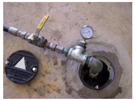
Photo No. 7. View of injection pump hose connection with pressure gauge and control valve.
