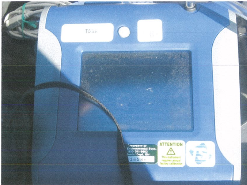
13. Dust Track monitor model 8530 used onsite.
