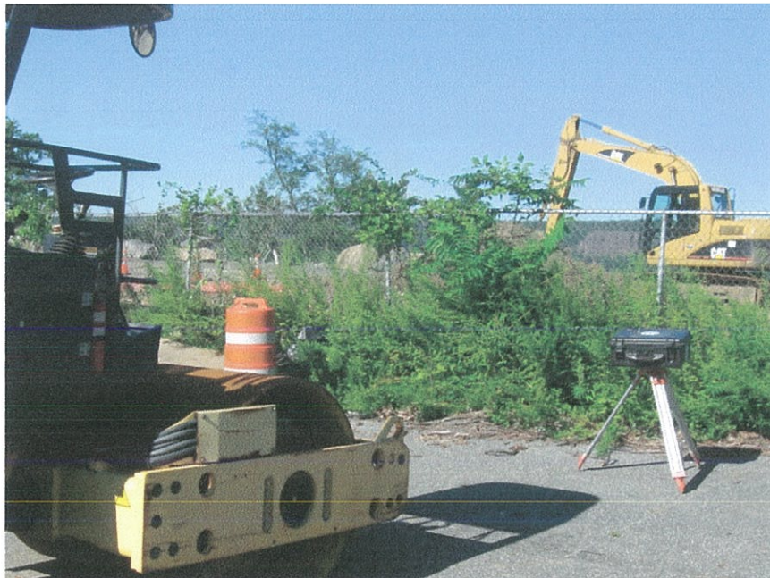
9. Downwind dust monitor as set-up.
