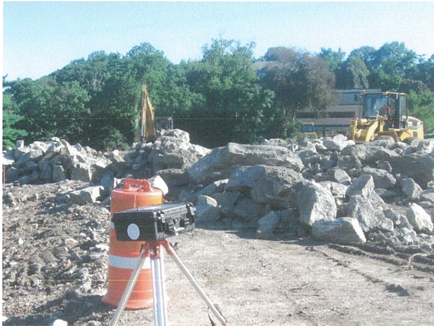
7. Upwind dust monitor as set-up.
