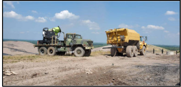
Portable odor and dust neutralizing systems
