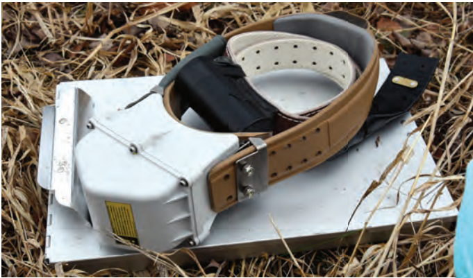
Biologists use radio collars like this one to help track a bear's movements.
