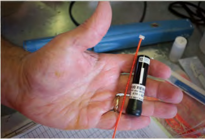
Scientists surgically implant AA-battery sized acoustic telemetry devices in selected lake trout to track and record their movements around Lake Erie.
