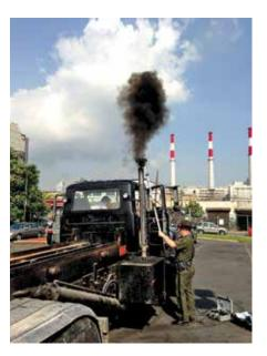
stopped the vehicle, and conducted a safety check and smoke meter test. The old truck failed the smoke meter test and the driver was issued a summons for exhaust over the opacity limit.
