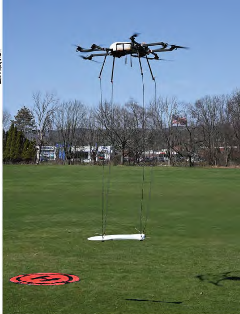
DEC's hybrid gas and electric octocopter carrying the magnetometer.
